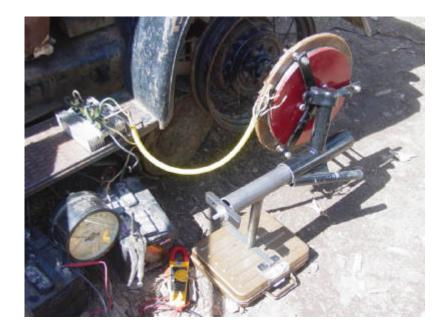
DanB's alternator dyno-testing rig
