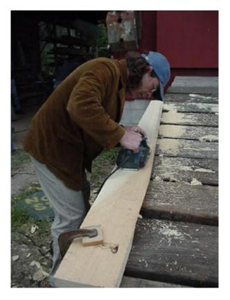
DanB running the planer on a blade for the new 12-foot machine design. The blades are Yellow Cedar, which cuts pretty well with a drawknife...but the turbine blades are BIG and the planer did speed up the process somewhat.
