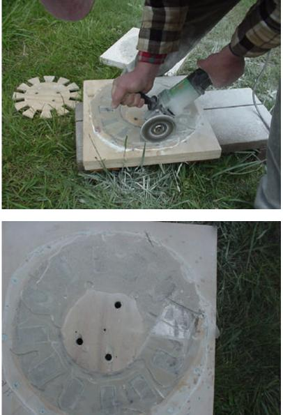
The operation was a success! The magnets we used were even saved intact, and could be re-used.
