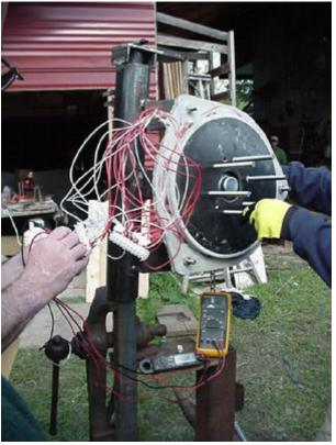
Assembling and testing alternator for 12-foot wind turbine. Note that each coil lead runs to external terminal blocks for future testing and R and D.
