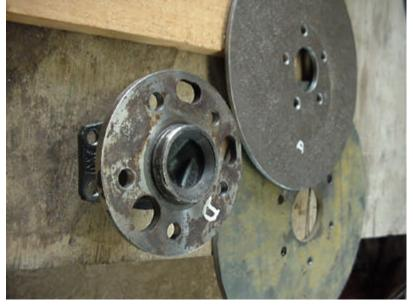
Note the perfectly circular magnet rotors, pre-drilled with perfectly spaced holes to fit the bearing. Well worth the money versus cutting these out with a torch and grinding them to perfection! These were from the 2004 seminar.
