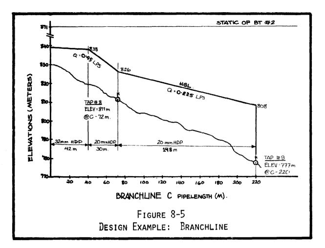
Branchline "C", First Reach (B'point - Tap #8) Design flow: (flow for 2 taps) 0.45 LPS 72 - 0 = 72 meters Pipelength: 839m (elev of HGL @ b'point) (elev of Tap #8) -811m (desired RH @ Tap #8) -15m 13m **DESIRED HEADLOSS**  $13/72 \times 100\% = 18.1\%$  desired frict'l factor A combination of 32mm HDP and 20mm HDP pipes is needed: 42m of 32mm HDP @ 2.56% creates 1m of headloss 30m of 20mm HDP @ 40% creates 12m of headloss actual residual head = 15m (perfect!)
