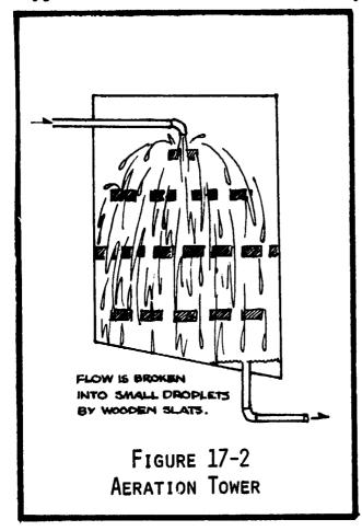
dissolved carbon dioxide) and reduces undesirable tastes and colors due to the presence of iron or other dissolved gases.
