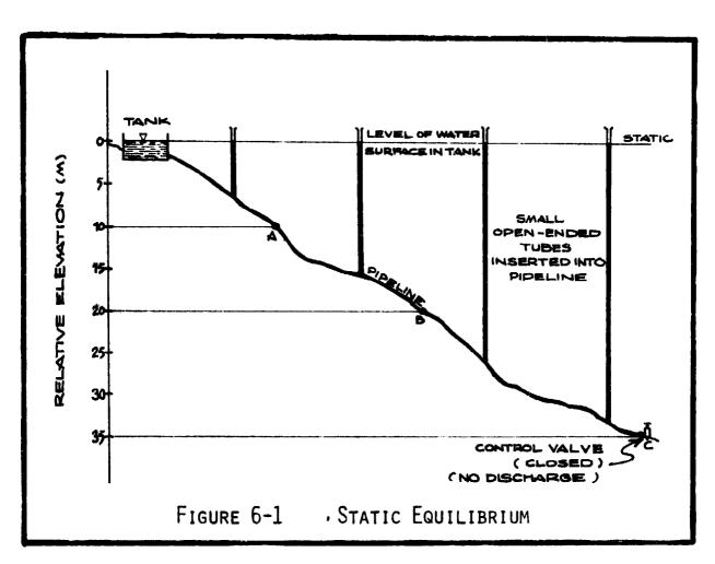
In a pipeline where no water is flowing, the system is termed being in <u>static equilibrium</u>. In such systems, the level of the water surface is called the <u>static level</u>, and the pressures are reported as <u>static heads</u>.
