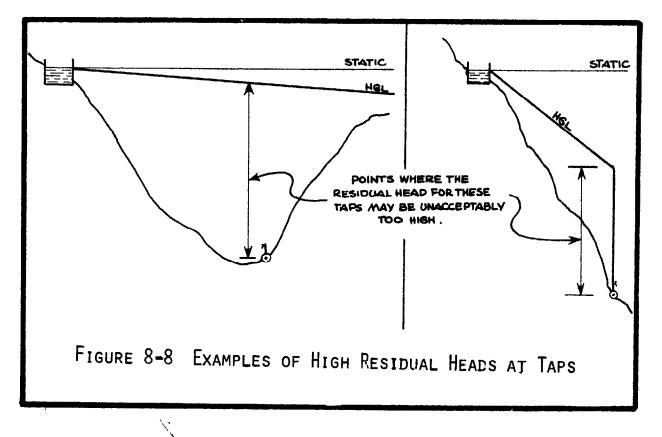
For such cases, it is possible to install a device which creates high frictional losses in only a short length of pipeline. This sort of frictional diffuser can be easily manufactured in the field, using HDP pipe and fittings. A design for this is shown on the next page.
