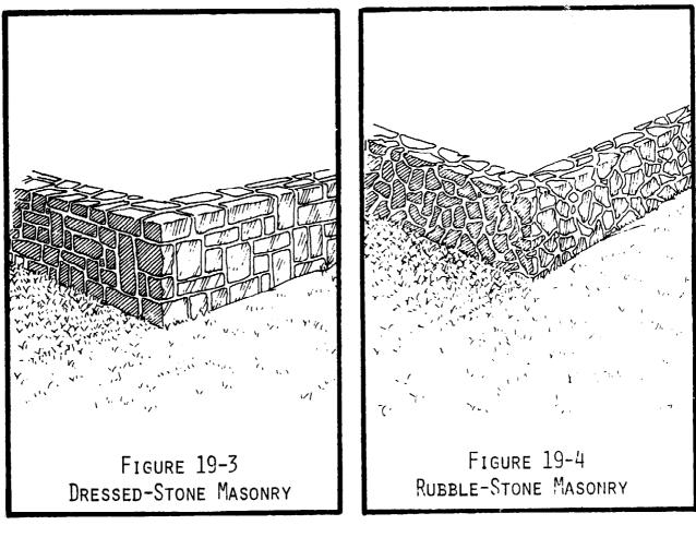
time and labor. Ashlar masonry is approximately 30% mortar and 70% stone. Refer to Figure 19-3:
