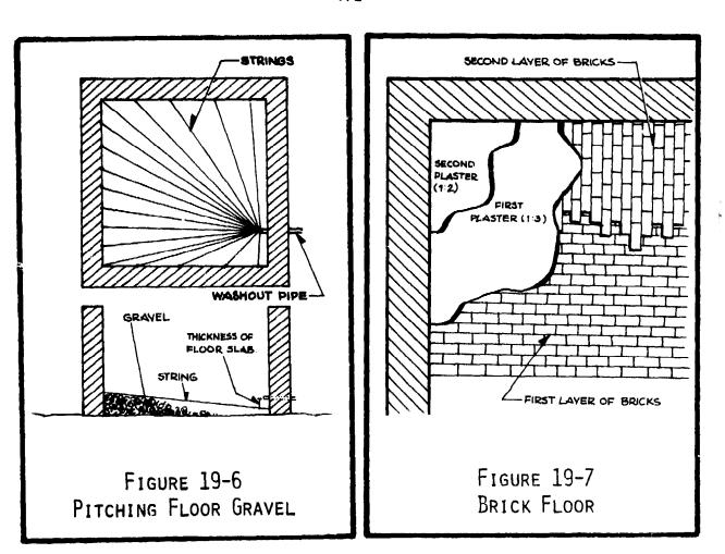
no spatterdash coat needed). As soon as the second plaster coat has set, the tank should be flooded a few centimeters deep (for curing the mortar) for several days. Refer to Figure 19-7.
