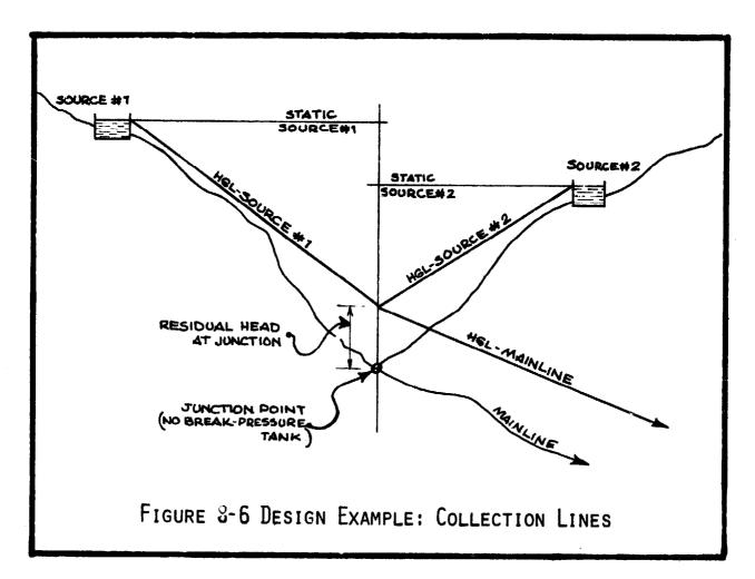
With this type of junction, if the sources are at different elevations then it is possible that the pressure from one will interfere with the flow from the other.
