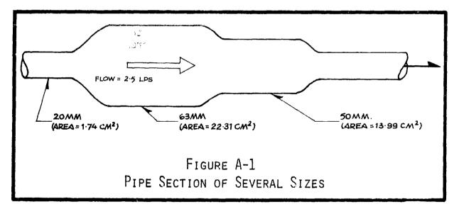
Knowing the flow (2.5 LPS =  $2500 \text{ cm}^3/\text{sec}$ ) and the cross-sect'l areas of the pipe sizes, the Equation of Continuity can be used to calculate the velocity of the flow through each pipe size:
