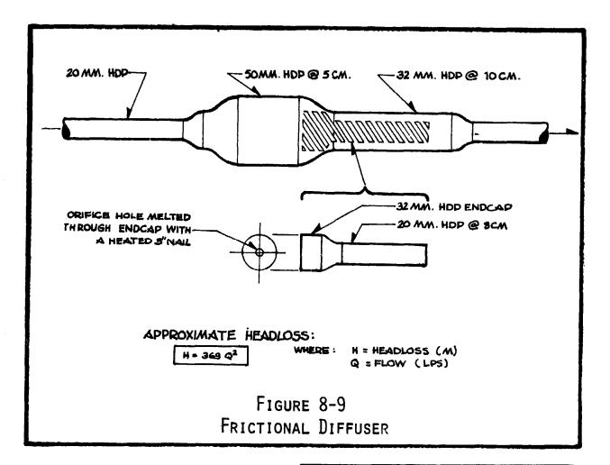
The orifice in the endcap is made using a hot 3" nail to melt a hole. For a flow of 0.225 LPS, this diffuser will create approximately 20-25 meters of headloss. Adding more holes <u>decreases</u> the headloss; if the headloss of a single diffuser is not enough, add a second one. The pipe section must be of Class IV HDP if the diffuser will be subjected to a static pressure greater than 60 meters of head.
