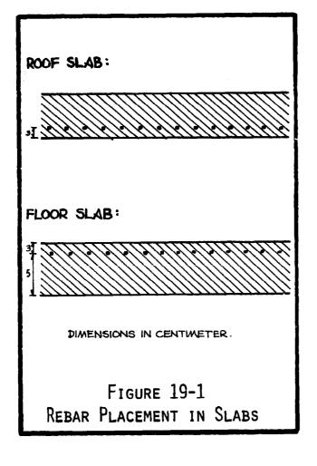
tied together with thin wire or string. The rebar must have a minimum of 3 cm of concrete covering. For a roof slab, the rebar is set 3 cm from the <u>bottom</u> of the slab, and for a floor slab the rebar is set 3 cm from the <u>top</u> of the slab (Refer to Figure 19-1).
