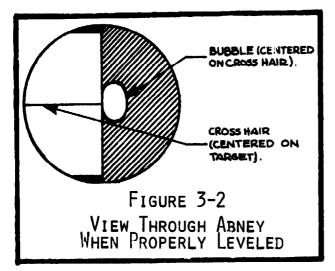
all aligned horizontally, as shown in Figure 3-2. The angle of view (technically known as the <u>vertical</u> <u>angle</u>) is then read on the arc in degrees.
