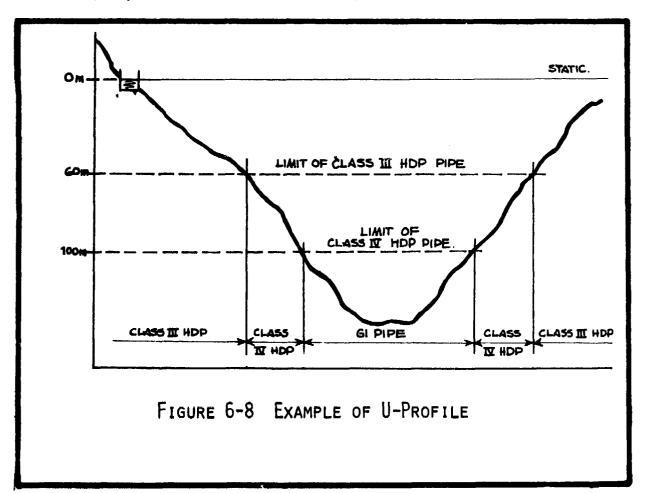
It is apparent from the figure above that, under static conditions, the pressures in U-profiles can be quite high. Sections where the pressures exceed 60 meters of head will require Class IV HDP pipe, and where there is more than 100 meters of head GI pipe will be required.
