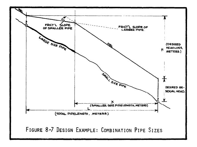
Since the total pipelength, design flow, and desired headloss are all known, the lengths of the two pipe sizes can be determined by the following equation:
