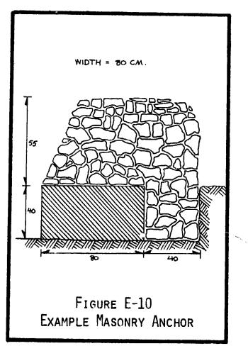
Designing the masonry block anchor (east bank)
