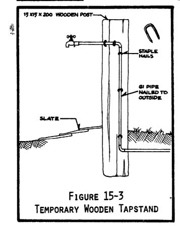
tapstands, due to the moist environment which promotes rotting. However, occasionally some projects will temporarily require such tapstands until cement can be obtained to build the proper one. In such cases, a wooden post, 15cm square minimally by 100cm longer than the height of the faucet, can be quickly installed. The village blacksmith is able to make a few iron staple-nails with which the GI pipe can be firmly nailed to the post. This type of tapstand is shown in Figure 15-3.
