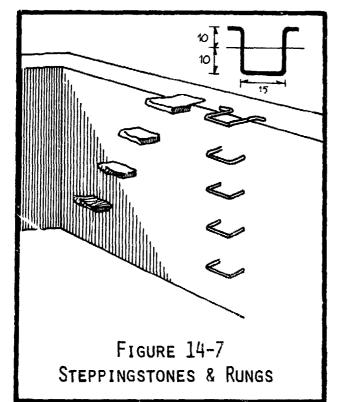
below where the accessway is to be located (refer to Figure 14-7). The rungs can be easily fashioned by the village blacksmith, to the dimensions shown in the figure. Rungs or steppingstones should be spaced 30 cm apart vertically. Refer to Chapter 19 for details on cement, mortar, and masonry.
