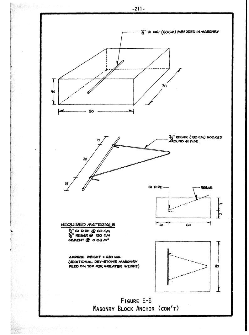
The total weight required is governed by the type of soil that the anchor is imbedded in, and the angle of the suspension cable. Different soils have different frictional characteristics:
