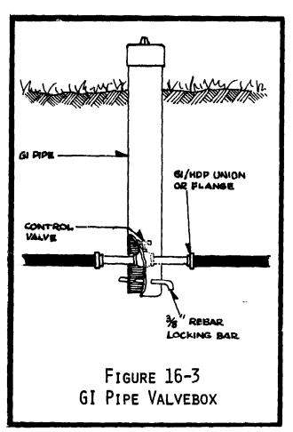
for a single valve, it is possible to use a length of GI pipe as the
