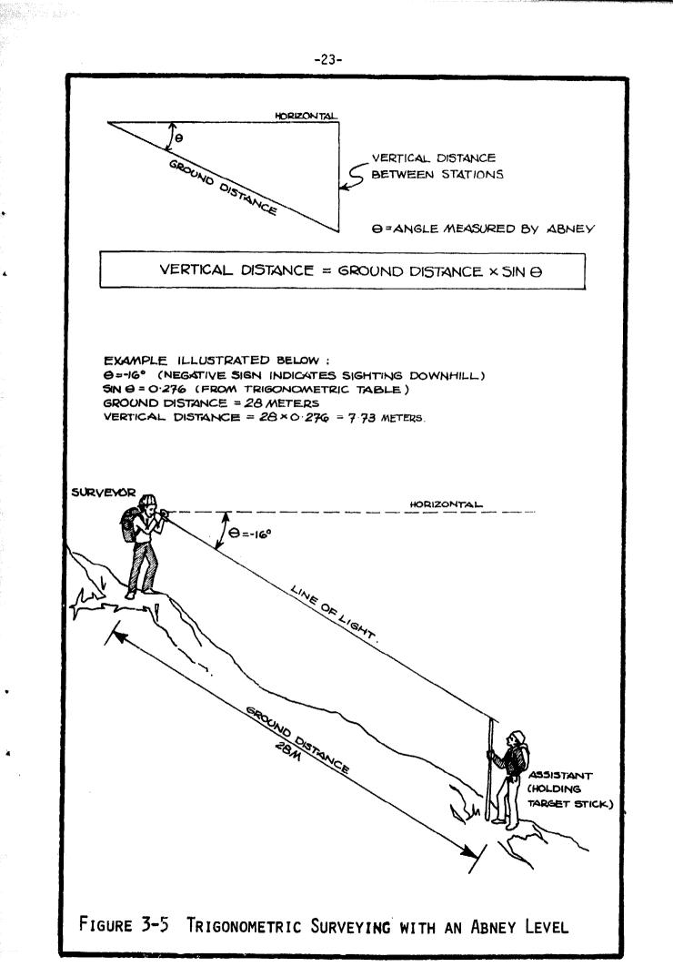
angle indicates that the surveyor was sighting downhill). By consulting a table of natural sines and using trigonometry, it is possible to calculate that the vertical distance between them is 7.7 meters. The reference tables at the back of this handbook present the natural sines, and also the elevation changes for various ground distances and vertical angles.
