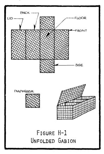
and can quickly instruct other villagers how to make the gabion cages.
