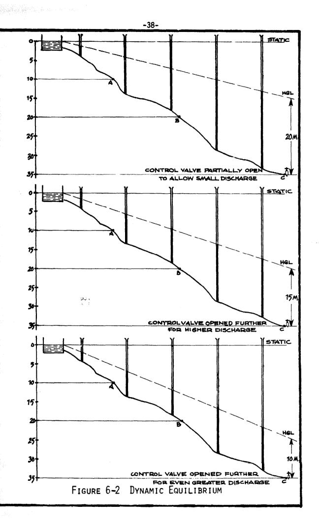
It can be seen that the water heights in these tubes form a new line for each new flow through the system. For a constant flow, the line formed by the water heights will remain steady. The system is now said to be in <u>dynamic equilibrium</u>. The line formed by the water levels in the tubes is called the <u>hydraulic grade line</u>, commonly abbreviated as HGL. A different flow establishes a different dynamic equilibrium, and a new HGL.
