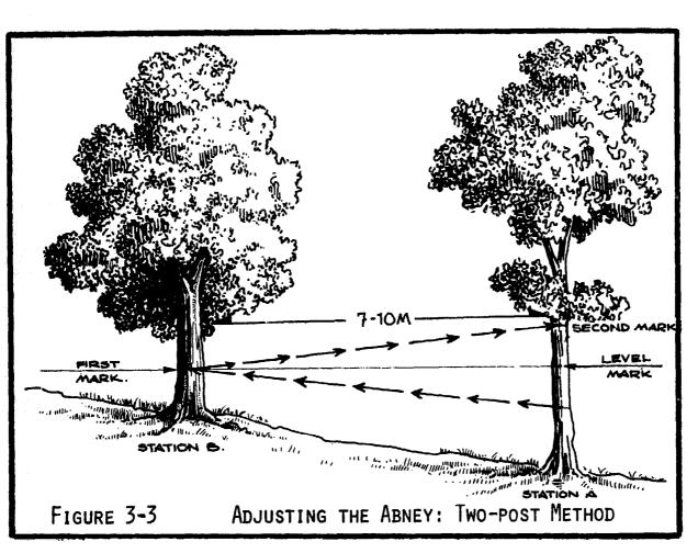
Many surveyors set up permanent level sight lines in their offices or on convenient outbuildings, so that it is only the work of a moment to check the Abney and adjust it themselves (not needing an assistant at all).
