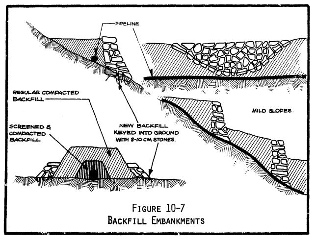
Steep slopes: Where the trench cuts down a steep incline, the backfill is vulnerable to easy erosion by rainfall, which will tend to wash all backfill to the bottom of the slope. Facing the trench with stone, as shown in Figure 10-8, will
