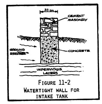
This is the component where the source flow is captured. In a spring intake, it is typically watertight walls surrounding the source point.
