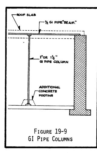
Figure 19-9 shows the arrangement of a GI pipe column and beam.
