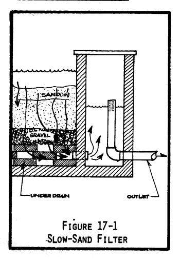
A slow-sand filter is a large tank that has an under-drain system which is covered by a base layer of gravel and then a bed of filtering sand. The filter works by mechanically straining the water as it flows through the sand, and also by biologically attacking the organic impurities (the filter bed develops a "slime" of bacteria, which feed upon the organic impurities carried in the flow).
