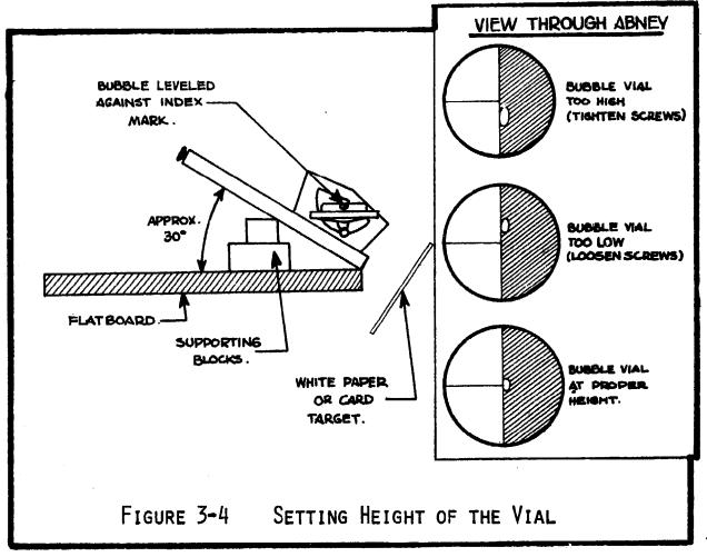
Hold a white card in front of the tube and sight through the instrument. The bubble should be centered on the cross-hair. If it is not, adjust the height of the bubble level by tightening or loosening the mounting screws equal amounts in the <u>same</u> direction. If the bubble appears too low, then lower the level by tightening the screws, and vice versa.
