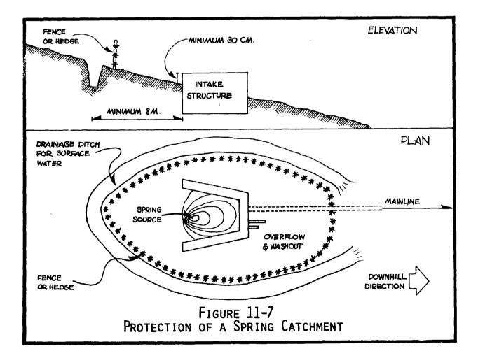
above ground level. Dirt should be mounded against the tank walls so that water will be turned away, and the source should have a drainage ditch dug around its uphill side. This channel should be deep, and can be lined with dry-stone masonry. Each year, particularly just before the monsoon season, it should be cleared of accumulated debris. The catchment of a spring source can be roofed over with a concrete slab, and buried for further protection.
