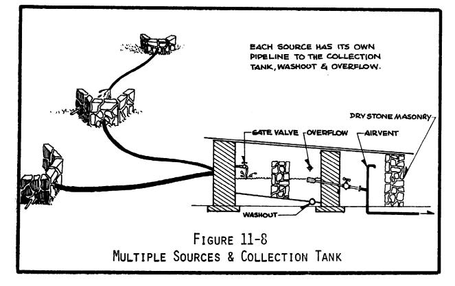
by the distances and elevations between the sources. Flow from higher sources can be piped directly into lower sources, or each source may have its own individual pipeline to a single collection tank or sedimentation tank. Each catchment requires its own washout and overflow pipes, but a gate valve can be located at the discharge point into the collection tank. It is not necessary that each catchment have its own settling chamber, so long as the total flow has the opportunity to settle.
