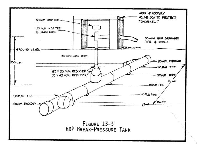
The rate of flow out of the HDP break-pressure tank will be dependent upon the head of water acting at the outlet pipe. This head will be limited by the height of the snorkel overflow tee above the outlet pipe. Consequently, the HDP break-pressure tank should be at least one meter below the overflow tee, i.e. about 90cm below ground level.
