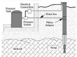
feet extending into the bedrock. The casing should also extend a foot or two above the ground's surface. A sealant, such as cement grout or bentonite clay, should be poured along the outside of the casing to the top of the well. The well is capped to prevent surface water from entering the well.
