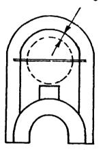
Complete upper vault leaving a 3 - 5 cm gap between the bricks and the drum.
