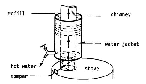
A simpler device is used in Africa. The metal chimney pipe is surrounded with a jacket, which is filled with water. A tap is fixed at the bottom to drain the heated water. The system will provide good service for warm water, however, one has also to consider that one can not extract all the heat in the smoke for heating the water (otherwise the gases may condense and soot be deposited in the chimney).
