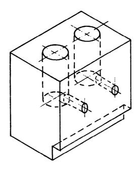
This second model is loaded with the help of two sticks or pipes. One is first pushed through the front opening at least as far as the center of the stove, and the other is held upright resting on the horizontal pipe. Then the unit is packed with sawdust and both pipes or sticks are drawn out. To light this stove, the paper is shoved in horizontally.
