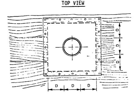
To prevent heat transfer from the pipe to the ceiling materials a space, all around the metal pipe, of the diameter of the pipe (or even with more distance) is required.
