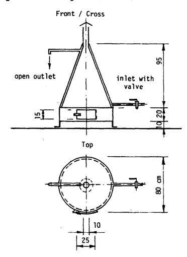
It was a double cone of galvanized-iron sheeting, one inside the other, with a gap of two or three millimeters between them. Water entered at the bottom and came out at the top. The cone was mounted on a fire box in which old newspaper were crumpled up and set ablaze. Within a few seconds the outflowing water was hot. Once the fire is lighted, the water should be allowed to flow, or steam pressure may build up and burst the cone.
