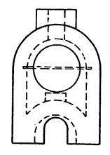
Use mud plaster to close in the front of the oven up to the drum. Use drum lid as a door. Build chimney extension.
