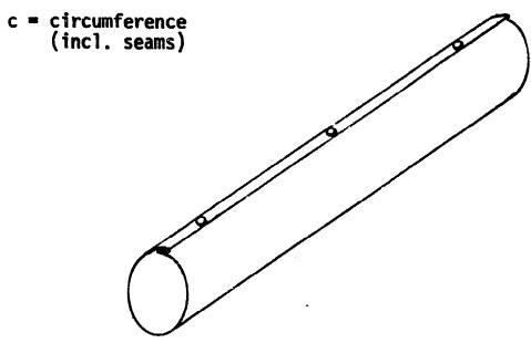
Sheet metal pipes may be riveted or folded. If folding is applied some rivets are required to prevent the seams' opening.
