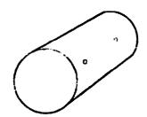
Drill holes in drum for support rods (ID - 12 mm). These rods help to stabilize the drum and hold the tray for the upper row of bread pans.
