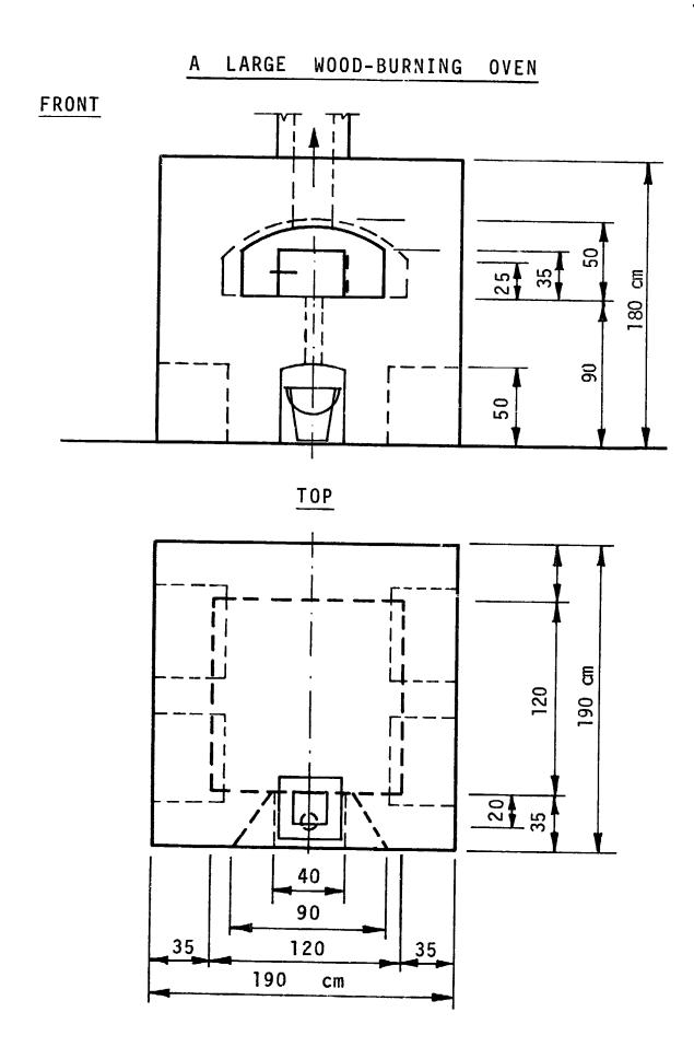
That is the basic design of the oven. A few helpful improvements are recommended. The thin metal sheet covering the ledge could be replaced by an iron plate, say 2 mm thick, of the same shape, hinged along the front edge so that it can be flipped up to expose a hole in the ledge through which the embers can drop straight into a bucket recessed into the oven wall. This is neater and cleaner than letting the hot embers and ashes fall on the floor.
