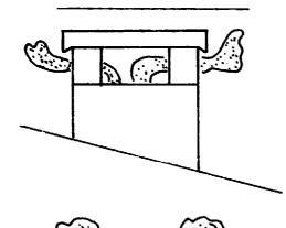
The top of a chimney requires a hat for protection from rain. However, the design may need to to be in such a way that the draught is increased, even with wind from the side (without providing back-flow to the stoves.
