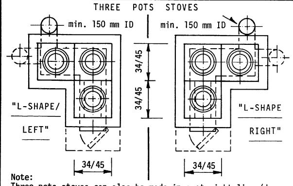
Three pots stoves can also be made in a straight line (in the same way as the two pots stoves). The third hole serves mainly for lower temperature cooking.
