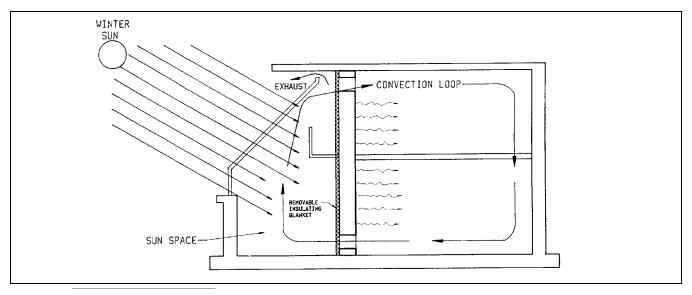
Figure 2. Isolated gain system using a sun space
