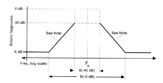
Figure 2. Radar Emission Bandwidth and Emission Levels
