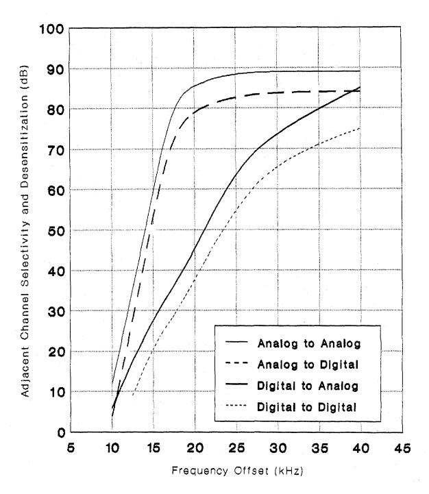
Figure 10. Adjacent Channel Selectivity and Desensitization
