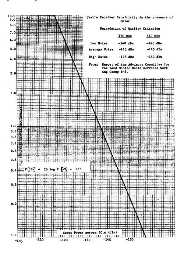
Figure 1. Voltage to Power Conversion
