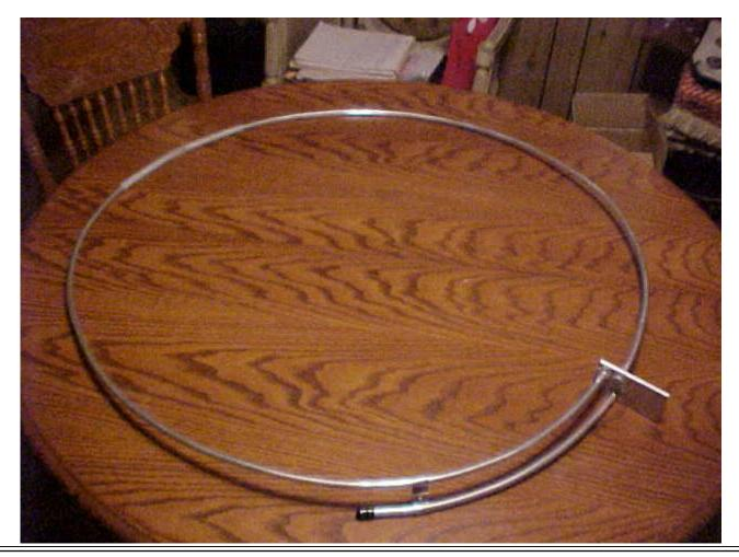
Both 54" elements are bolted and welded to the mounting plate. Use galvanized or some other type of corrosion resistant bolts. The size of the bolts is not so important other then that they fit snugly into the ends of the 3/8" fu line and hold the elements in place while welding the elements to the mounting plate. This "Alumalloy" product great for this purpose and is more like soldering than welding. After the 2 elements are welded, leave the 2 bolts place for added support.
