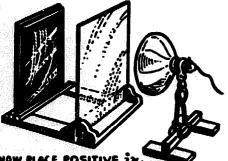
HOW PLACE POSITIVE IN SAFE-EDGE SIDE TOWARDS LAMP. PLACE & PIECE OF CARDBOARD OVER BACK OF POSITIVE TO PREVENT LIGHT REFLECTION FROM PENETRATING INTO BACK OF TISSUE DURING EXPOSURE. EXPOSE IS MIN. of 30 IN. with N°2 PHOTO FLOOD LAMP, or 15 MIN. of 40 IN. with CARBON ARC LAMP.
