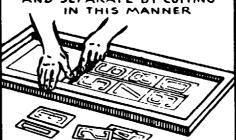
NOW MAKE ANOTHER SCREEN 3 USING 8XX MULTIFILAMENT FABRIC WITH AN OPENING AS SHOWN BELOW, FOR THIS YOU CAN USE CUT FILM, OR HAND FILLED.
