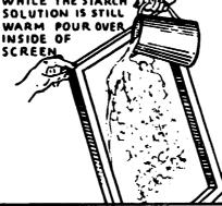
AFTER STARCH IS DRY ON SCREEN, THEN USE A BLOCK OR OTHER MEANS FOR A SUPPORT, SAME THICKNESS OF SCREEN FRAME AND PLACE INSIDE
