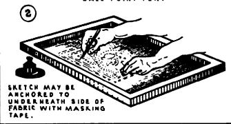
THE SCREEN IS THEN PLACED IN AN UPRIGHT SLANT-ING POSITION, OR BRIDGE MAY BE USED AS SHOWN IN INSERT OVER ILLUMINATED GLASS TABLE TOP. TUSCHE IS THEN APPLIED TO THE
