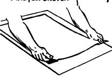
CUT THE THIN COATED VELLUM FILM AND PEEL AWAY, SAME AS WITH REGULAR CUTTING FILM
