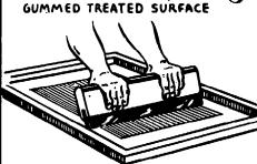
AFTER FIRST COAT IS DRY, THEN SQUEEGEE A SECOND COAT DRYING TIME OF EITHER COAT ABOUT ONE HOUR
