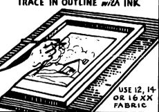
NOW FILL IN WITH BLOCKING-OUT LACQUER UP TO OUTER EDGE OF DESIGN THIS REMAINS PERMANENT USING RED SABLE BRUSH
