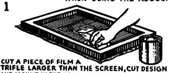
TRIFLE LARGER THAN THE SCREEN, CUT DESIGN AND MOUNT IN THE USUAL WAY, APPLYING SOLVENT TO FILM COMPLETELY INSIDE RIGHT UP TO FRAME
