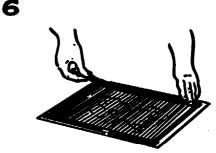
NOW TURN POSITIVE OVER SO EXACT EXE ATTACHED TISSUE is ON EXE UNDERNEATH SIDE and PROCEED to SAFE-EDGE with BLACK TAPE OVERLAPPING EDGE of TISSUE 1/2 IN.
