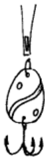
Lure made from a thrift store spoon: cut off the handle and file smooth.
