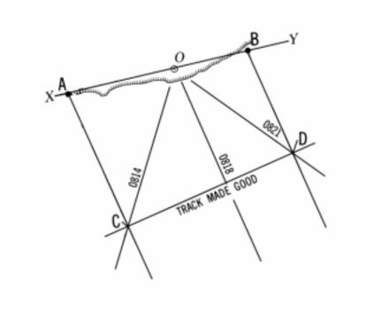
Figure 821b. Determining the track made good.
