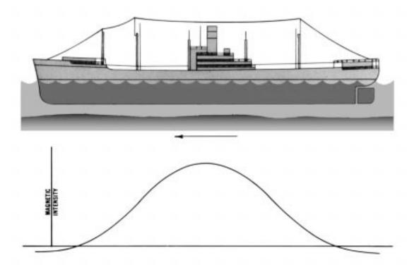
Figure 641b. A simplified signature of a vessel of Figure 641a.
