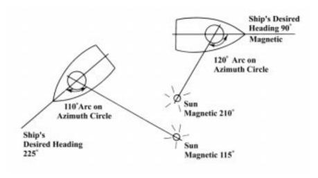
Figure 630. Azimuth circle set-ups.
