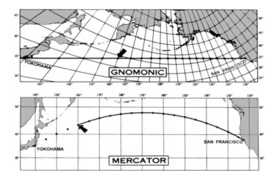
Figure 2501. Constructing a great circle track on a Mercator projection.
