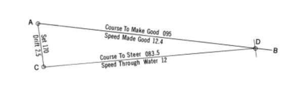
Figure 708b. Finding the course to steer at a given speed to make good a given course through a current.
