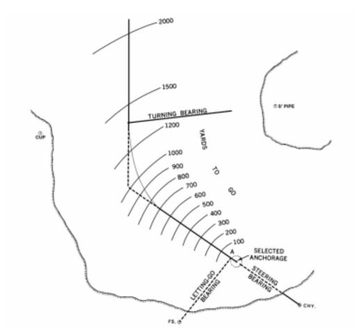
Figure 817. Anchoring.
