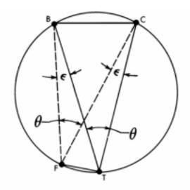
Figure 824b. Two-bearing plot with constant error.
