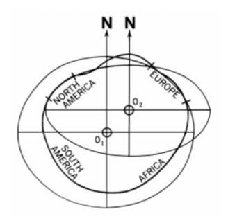
Figure 203. The geoid and two ellipsoids, illustrating how the ellipsoid which fits well in North America will not fit well in Europe, and must have a different origin.
