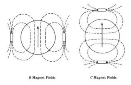
Figure 626b. Arrangements of corrector magnets.
