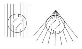
Figure 626a. Magnetic fields across compass needle arrays.
