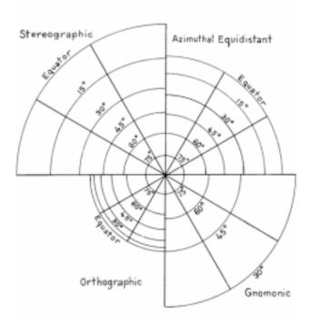
Figure 320. Expansion of polar azimuthal projections.
