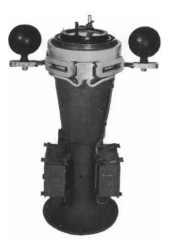
Figure 646. Type K degaussing compensation installation.
