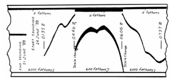
Figure 3016a. Properly annotated echo sounding record.
