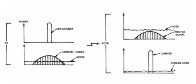
Figure 1106c. GPS signal spreading and recovery from satellite to receiver.
