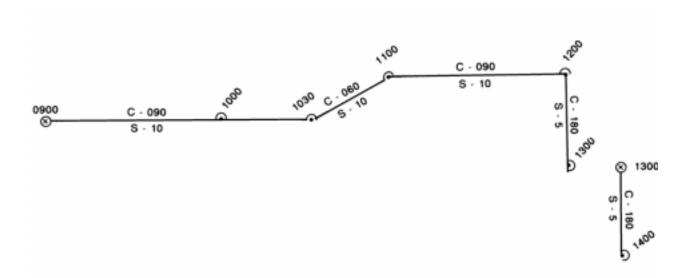
Figure 703. A typical dead reckoning plot.
