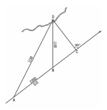
Figure 822. Triangles involved in a Table 18 running fix.
