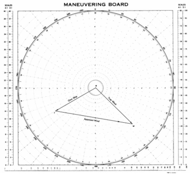
Figure 3710. Finding true wind by Maneuvering Board.
