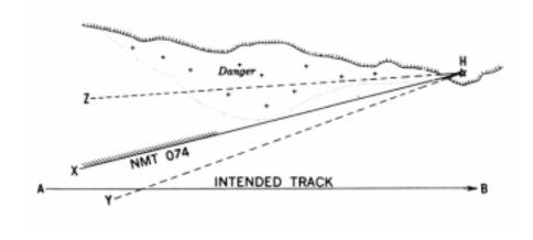
Figure 801d. A danger bearing, hatched on the dangerous side and labeled wih the appropriate bearing.
