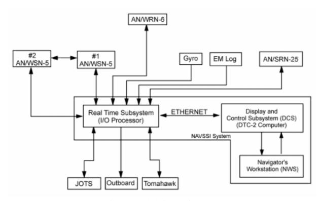
Figure 1410. Block diagram of NAVSSI.
