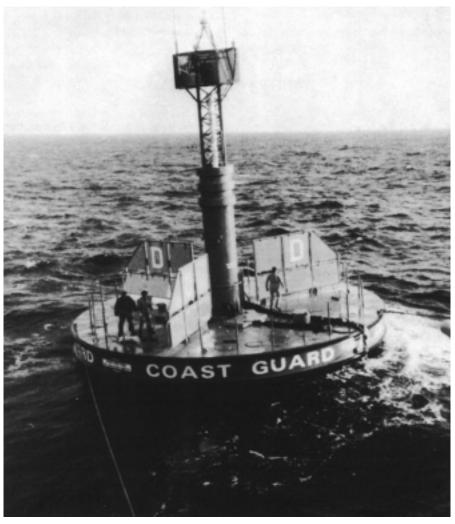
Figure 513. Large navigational buoy.
