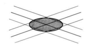
Figure 2304b. Ellipse of uncertainty with lines of positions of equal probable errors crossing at an oblique angle.
