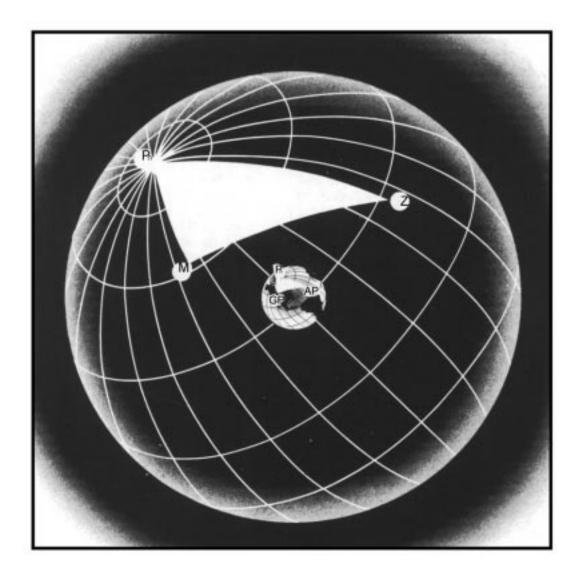
Figure 1530b. The navigational triangle in perspective.
