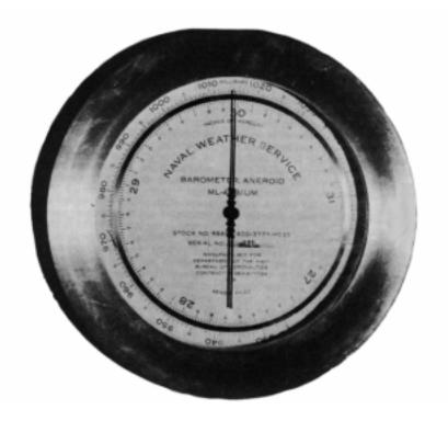
Figure 3703. An aneroid barometer.
