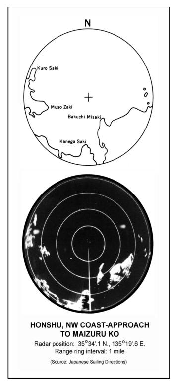
Figure 1302. Plan Position Indicator (PPI) display.
