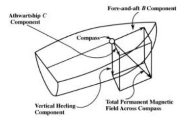
Figure 605a. Components of permanent magnetic field.
