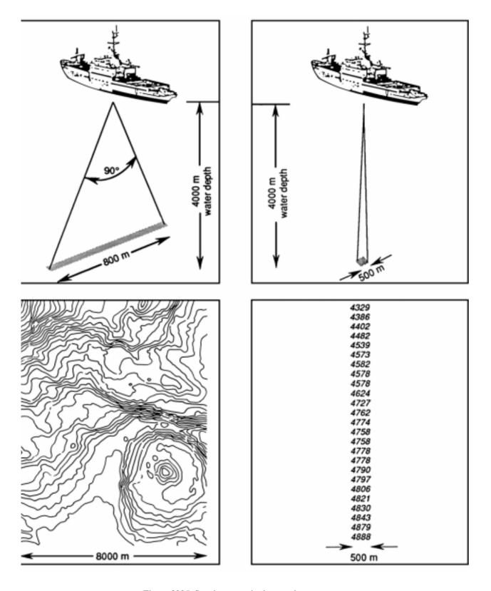
Figure 3005. Swath versus single-transducer surveys.
