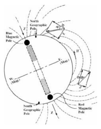
Figure 603a. Terrestrial magnetism.
