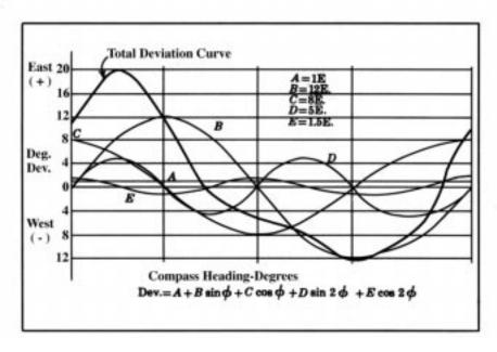
Figure 615. Example of typical deviation curve and its components.
