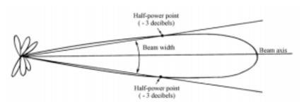
Figure 1303b. Radiation diagram.
