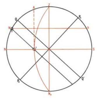
Figure 1529e. A diagram on the plane of the celestial meridian for lat. 45°S.
