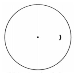
Figure 1307d. Second-trace echo on 12-mile range scale.
