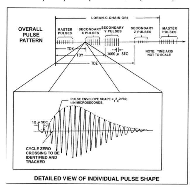
Figure 1205. Pulse pattern and shape for Loran C transmission.
