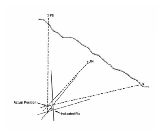
Figure 825. Adjusting a fix for constant error.
