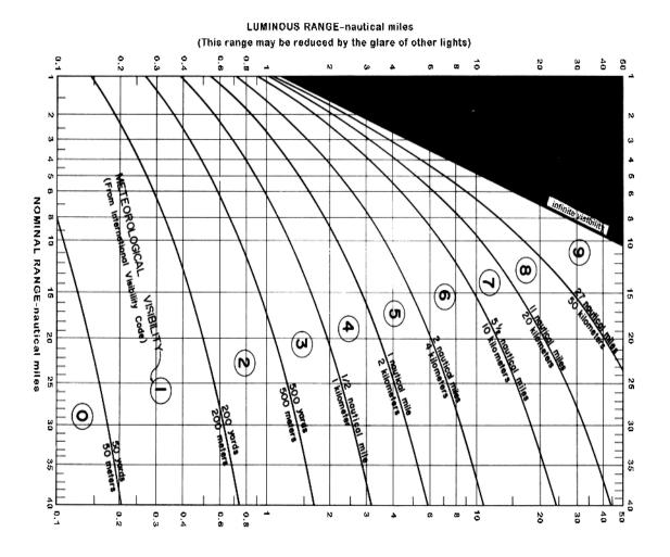
Figure 408a. Luminous Range Diagram.
