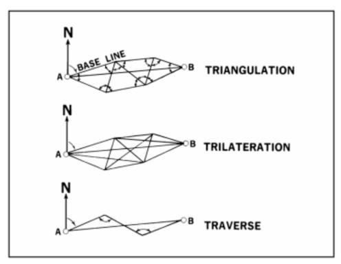
Figure 206. Triangulation, trilateration, and traverse.
