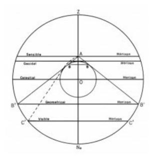
Figure 1526. The horizons used in navigation.
