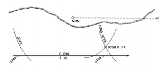
Figure 813g. A running fix by two circles of position.
