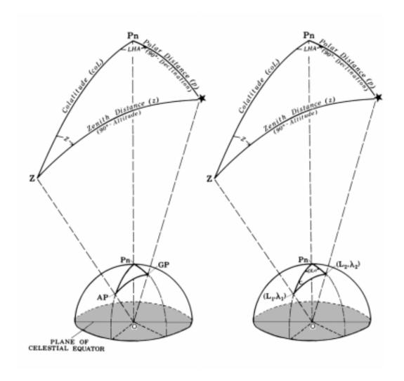
Figure 2405. Adapting the astronomical triangle to the navigational triangle of great circle sailing.
