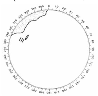
Figure 1308b. Coded racon signal.
