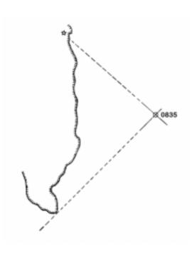
Figure 811a. A fix by two bearing lines.
