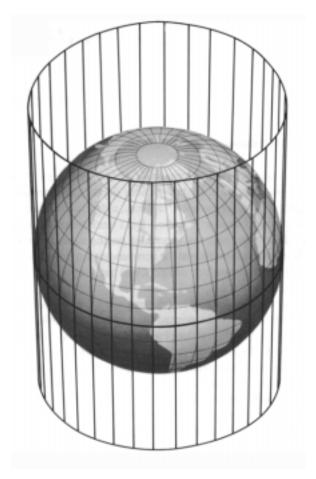
Figure 304. A cylindrical projection.
