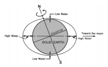
Figure 903c. Theoretical equilibrium configuration due to moon's differential gravitational forces. One bulge of the water envelope is located at the sublunar point, the other bulge at the antipode.
