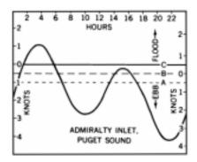
Figure 917a. Effect of nontidal current on the rotary tidal current of Figure 914a. If the the nontidal current is northwest at 0.3 knot, it may be represented by BO, and all hourly directions and speeds will then be measured from B. If it is 1.0 knot, it will be represented by AO and the actual resultant hourly directions and speeds will be measured from A, as shown by the arrows.
