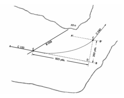
Figure 801b. Allowing for advance and transfer.
