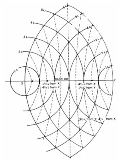
Figure 1214. Omega lanes formed by hyperbolic isophase contours.
