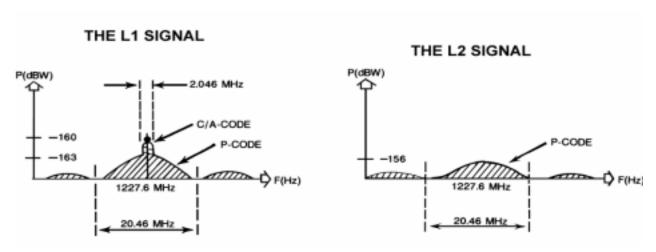
Figure 1106b. Modulation of the L1 and L2 carrier frequencies with the C/A and P code signals.
