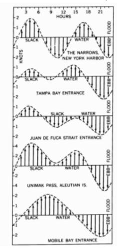
Figure 915a. Several types of reversing current. The pattern changes gradually from day to day, particularly for mixed types, passing through cycles.
