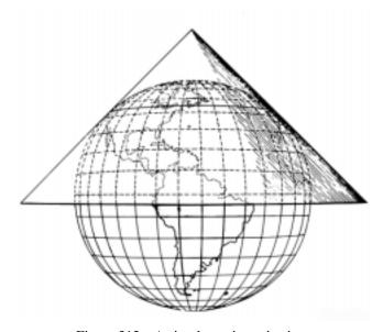
Figure 312a. A simple conic projection.
