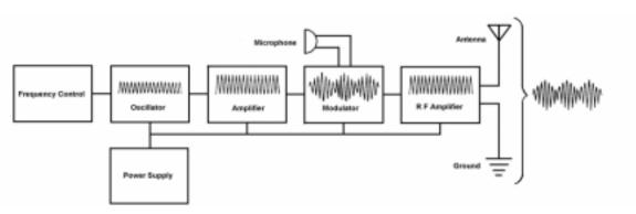
Figure 1016. Components of a radio transmitter.
