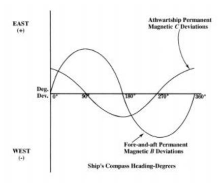
Figure 605b. Permanent magnetic deviation effects.
