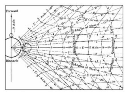
Figure 620. Slewing of quandrantal spheres.
