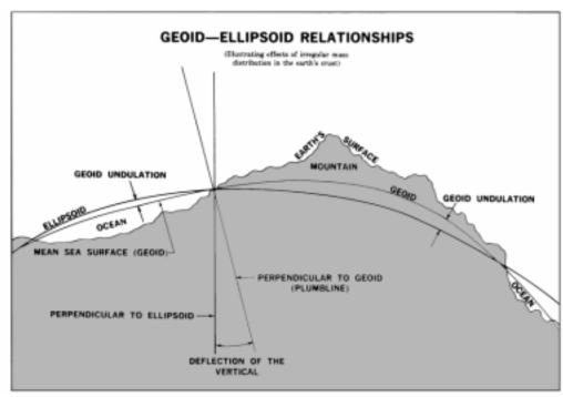
Figure 201. Geiod, ellipsoid, and topographic surface of the earth, and deflection of the vertical due to differences in mass.
