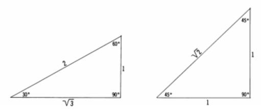
Figure 2108c. Numerical relationship of sides of 30°, 60°, and 45° triangles.
