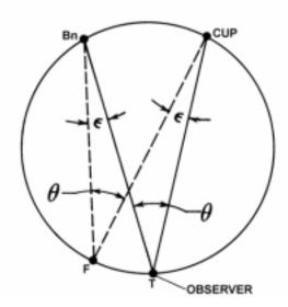
Figure 824a. Two-bearing plot.
