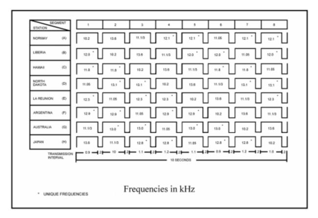
Figure 1212. Transmission format.
