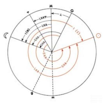
Figure 1525b. Time diagram. Local hour angle, Greenwich hour angle, and sidereal hour angle are measured westward through 360°. Meridian angle is measured eastward or westward through 180° and labeled E or W to indicate the direction of measurement.
