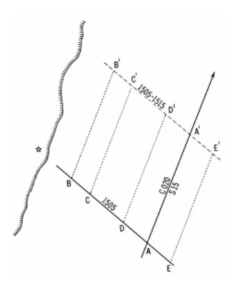
Figure 813a. Advancing a line of position.
