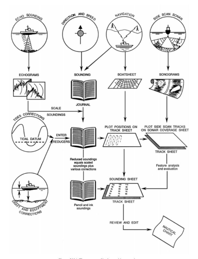
Figure 3004. The process of hydrographic surveying.
