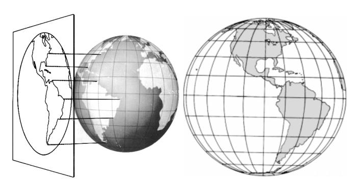
Figure 318a. An equatorial orthographic projection.
