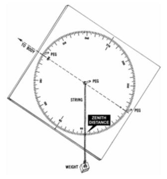
Figure 2608b. Improvised astrolabe; direct sighting method.
