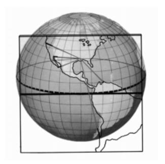
Figure 317a. An equatorial stereographic projection.
