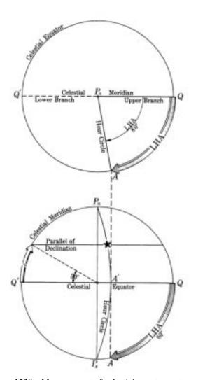
Figure 1529a. Measurement of celestial equator system of coordinates.
