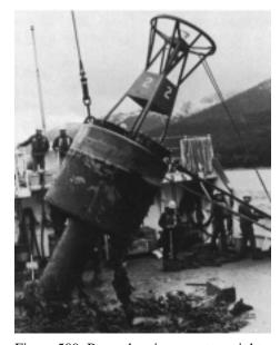
Figure 509. Buoy showing counterweight.
