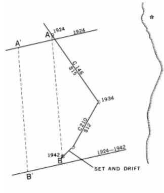
Figure 813b. Advancing a line of position with a change in course and speed, allowing for set and drift.
