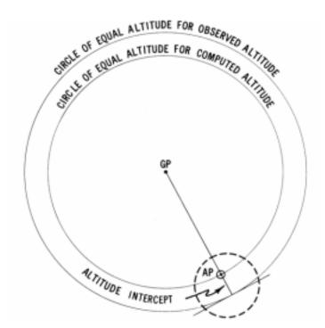
Figure 2003. The basis for the line of position from a celestial observation.
