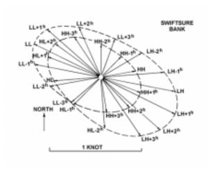
Figure 915c. Rotary tidal current with diurnal inequality. Times are in hours referred to tides (higher high, lower low, lower high, and higher low) at Swiftsure Bank.
