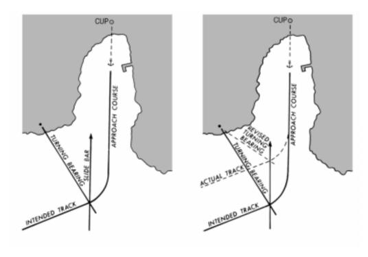
Figure 801c. The slide bar technique.
