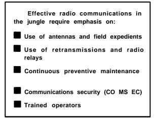
The usefulness of radio communications is reduced in jungle operations. VHF and UHF radios (FM radios included) are particularly limited by the jungle growth and terrain that absorb and obstruct the transmissions. It is not unusual for the range of a set operated in the jungle to be reduced by 10 to 25 percent of the normal range.
