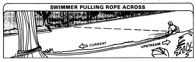
**One-Rope Bridge.** A one-rope bridge can be constructed either above water level or at water level. The leader must decide which to
