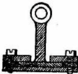
FIG. 64. — Cross section of crosshead and guide.
