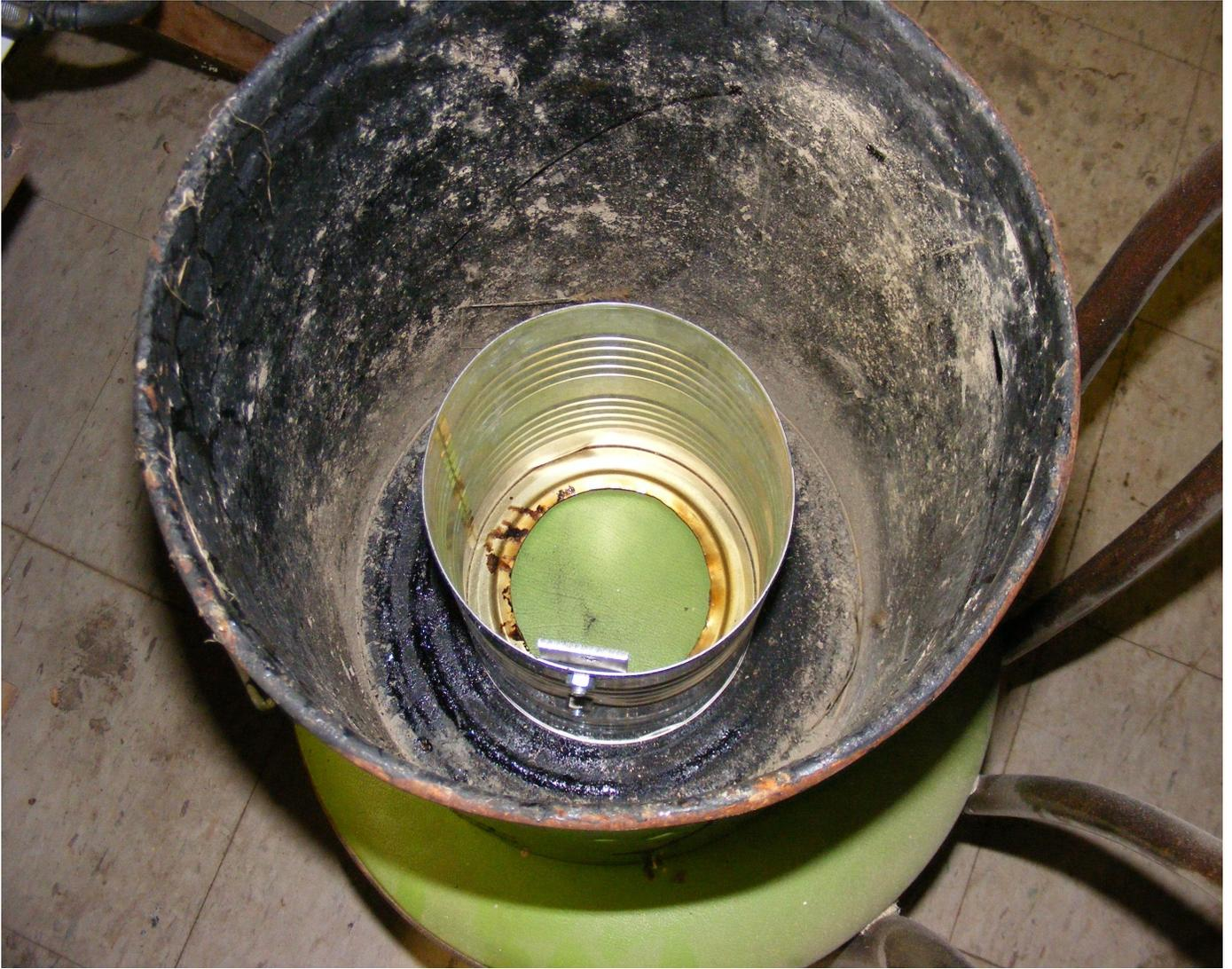
This is down inside the Bucket and the secondary air can. I will have to cut through both can to get the air pipe to the outside for the valve to connect.
