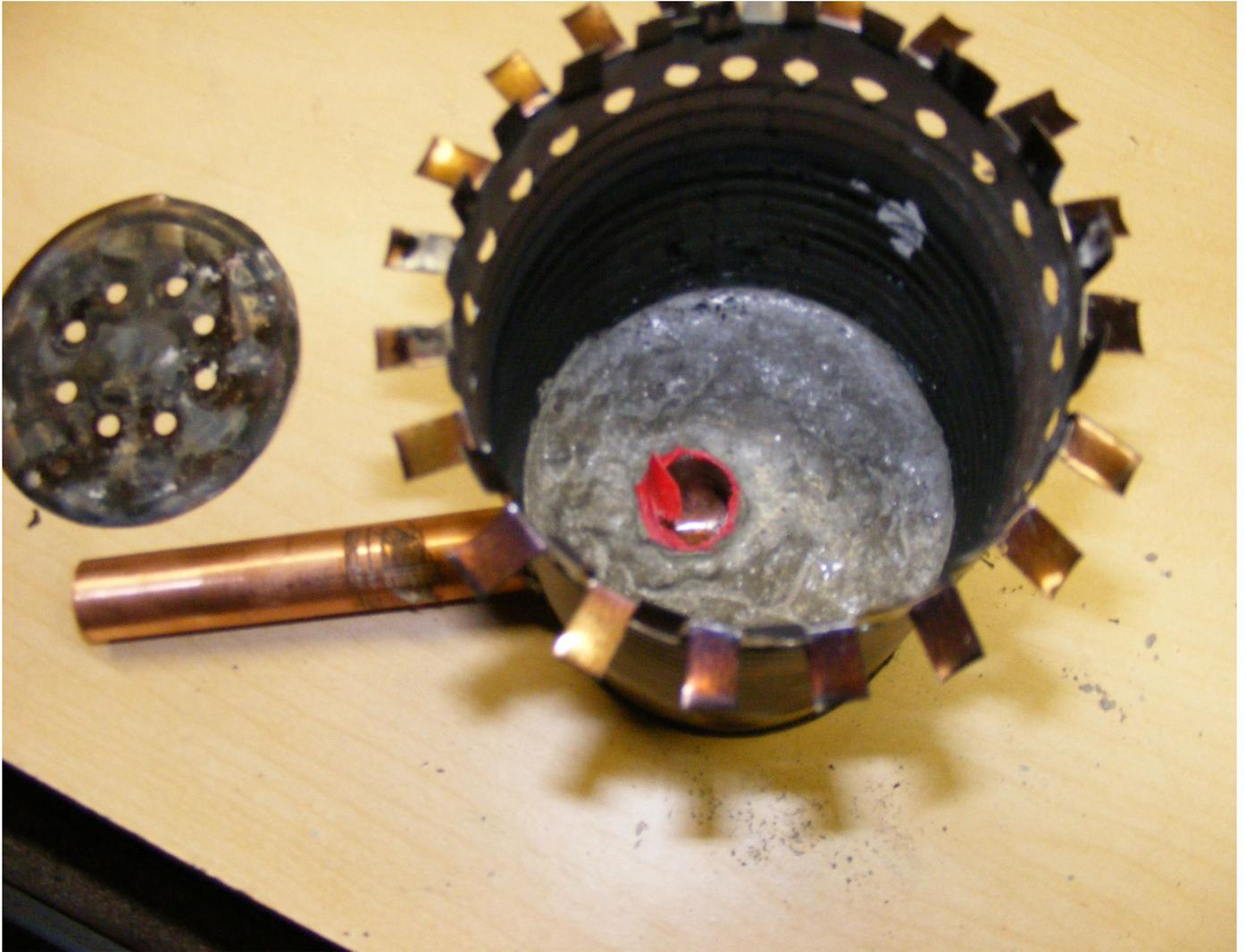
This is what it looks like down inside the burner. Tape is still ther but will be removed as it was used to cover the hole so no concrete would get inside.
