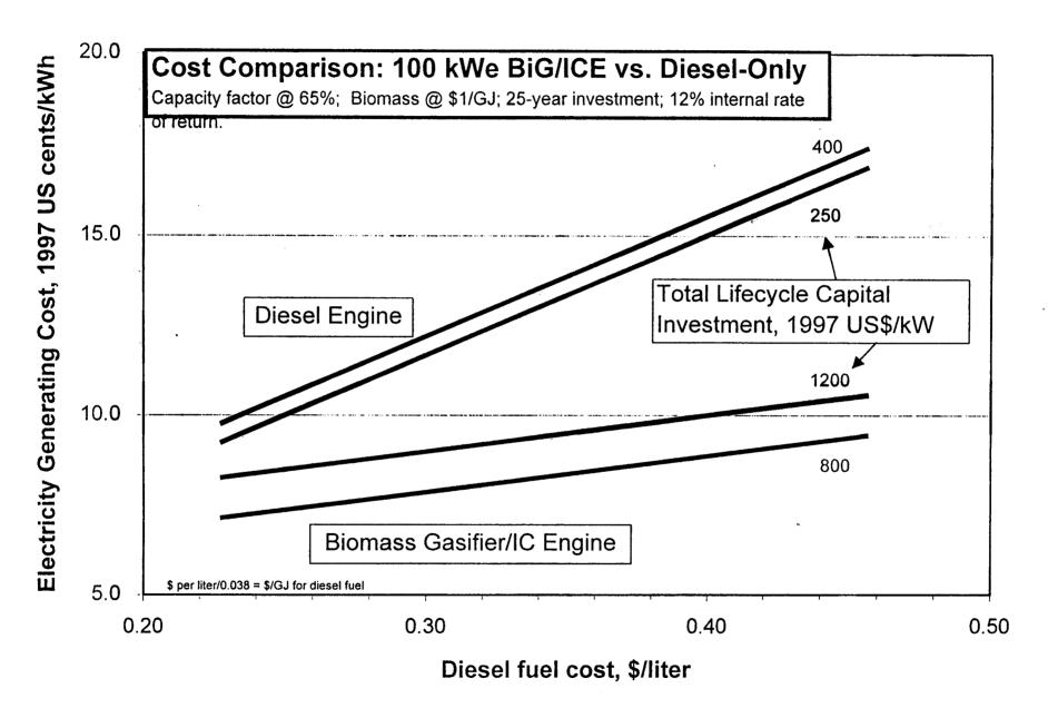
Fig. 12. Cost comparison between 100-kW<sub>e</sub> scale BiG/ICE and stand-alone diesel-only power generating systems as a function of diesel fuel cost.
