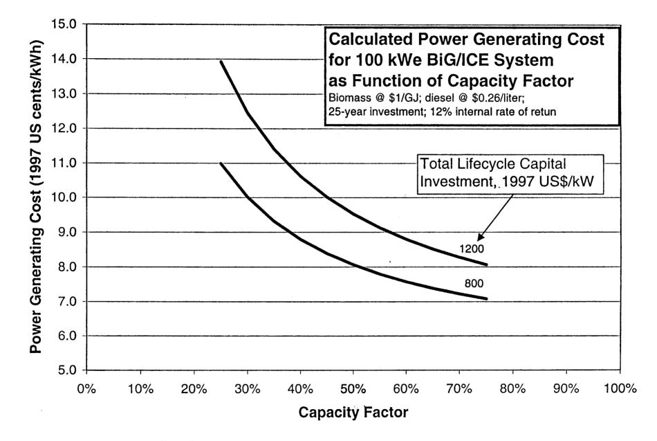
Fig. 13. Calculated electricity generating cost for 100 kW<sub>e</sub> BiG/ICE systems as a function of system capacity factor. Results are shown for two levels of initial capital investment. See Table 1 for additional details.
