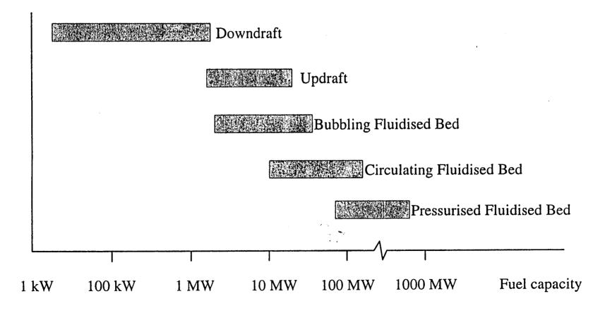
Fig. 4. Scales of application for alternative biomass gasifier designs. Source: TPS, Inc., Nyköping, Sweden.
