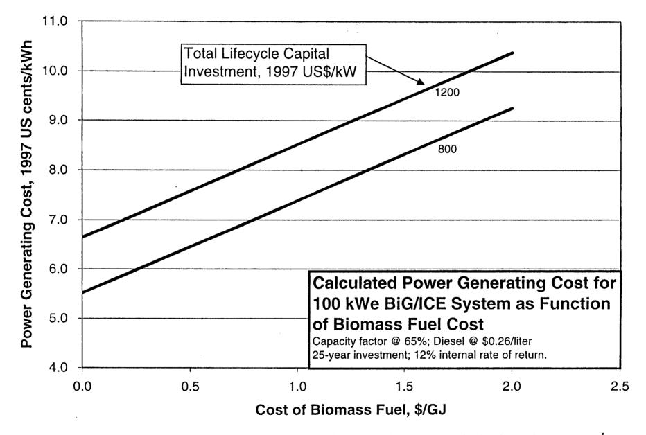
Fig. 14. Calculated electricity generating cost for a 100 kW<sub>e</sub> BiG/ICE system as a function of assumed biomass fuel cost. Results are shown for two levels of initial capital investment. See Table 1 for additional details.
