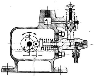
FIG. X.---38. Paxman Multiple-outlet Automatic Lubricator.
