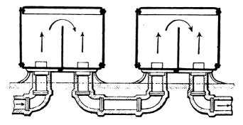
FIG. X.--52. Utilisation of waste heat in exhaust gases.
