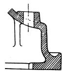
FIG. XII.-15. Boss for Foundation Bolt, with Stiffening Web.
