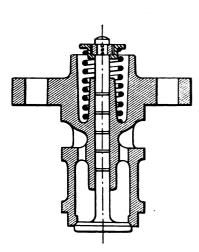
FIG. XIII.-79. Compression Spring on Inlet Valve.
