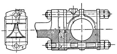
FIG. XIII.-24 and 25. Connecting Rod Head.
