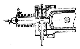
FIG. X.-28. Crossley Oil Engine Vaporiser with water injection device.
