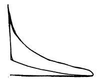
FIG. XI.—8. Indicator diagram showing violent explosion due to rich mixture.
