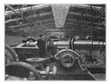
FIG. XIII.-19. Crank Shaft for 1,200 H.P. Nürnberg Engine.
