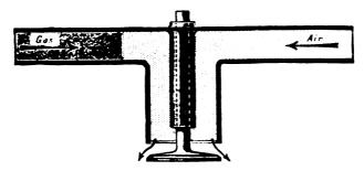
FIG. VIII.-5. Diagram showing Method of Supplying Air only at first opening of Inlet Valve (Koerting Engine).
