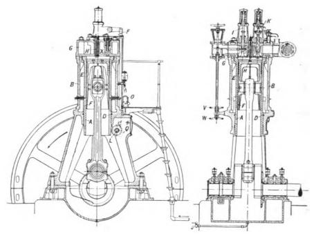
FIG. VI.--1. Sectional elevations of Güldner vertical Engine.
