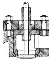
FIG. XII.—88. Removable Valve Seat with separate flange.
