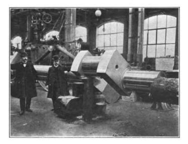
FIG. XIII.-18. Crank Shaft of 3,000 H.P. Nürnberg Engine.
