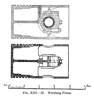
in the centre of the piston (Fig. XIII.—37). This arrangement was designed to protect the piston pin from the influence of high piston wall temperature, but appears to have been abandoned on account of its cost.
