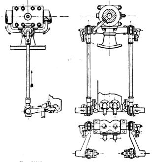
FIG. XIII.--48. FIG. XIII.--49. Koerting Water Cooling System to Piston and Rod.
