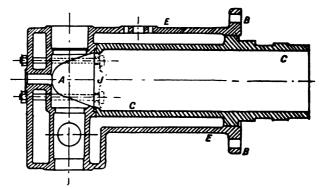
FIG. XII.-35. Liner in combined Combustion-chamber and Water-jacket.
