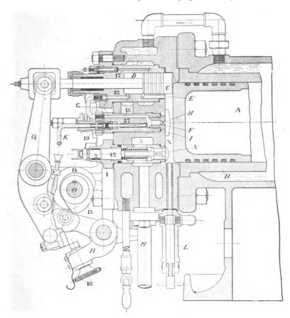
FIG. IX.-6.-The Trinkler (Koerting) Oil Engine.
