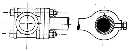
FIG. XIII.-26. Connecting Rod Ends.
