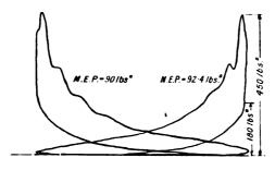
FIG. X.-50. Indicator diagram from double-acting Deutz Engine.
