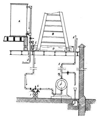
FIG. X. 35. Water circulation (closed system) with cooling apparatus.
