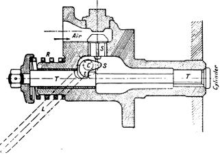
FIG. X -- 44. Tangye compressed air Starting Valve. Section.
