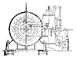
FIG. XII.-72. Koerting four-cycle Engine with side Valve Boxes.
