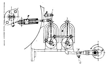
FIG. X.-22. Magneto mechanism, Koerting.
