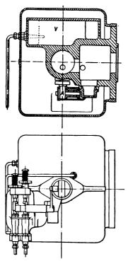
FIG. X.—31. Britannia Crude Oil Engine with water injection device.
