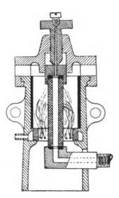
FIG. X.—7. Ignition device with porcelain tube.
