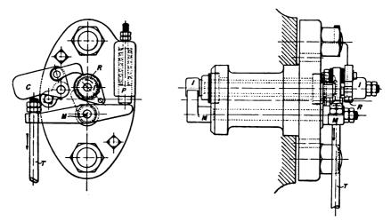
FIG. X.-24. Tangye self-cleaning Sparking points.
