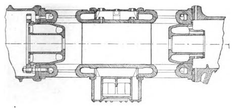
FIG. XII.-45. Section of Cylinder, Gasmotoren Fabrik Deutz.
