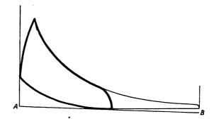
FIG. 1X.--3. Comparative indicator diagrams of Sargent and ordinary Four-cycle Engines.
