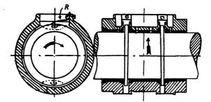
FIG. XII.-24. Bearing for Shaft with two fixed Oiling Rings.
