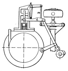
FIG. X1.-14. Gasmotoren Fabrik Deutz variable Valve Lift Device.
