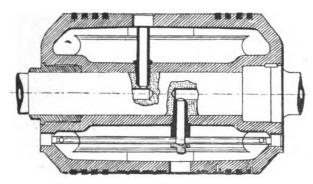
FIG. XIII.-50. Koerting water-cooled Piston.
