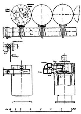
FIG. VI.-17. Mixture Regulation Device, Crossley vertical Engine.
