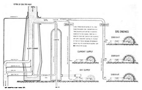
FIG. 1.-2. Thermal Balance Sheet of Blast Furnace of 250 tons per day capacity.
