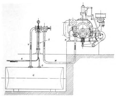
FIG. X.-46. Gasmotoren Fabrik Deutz compressed air starting equipment.
