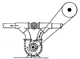
FIG. X.-33. Water circulation by Centrifugal Pump.
