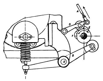
FIG. XIII.-70. Valve Gear with separate Cams.
