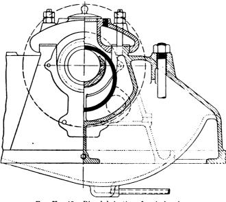
FIG. X.-42. Ring lubrication of main bearings.
