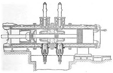
FIG. XII.-53. Section of Cylinder, Dingler.
