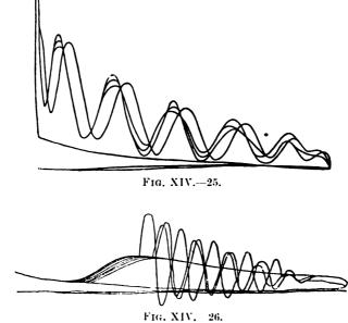
Undulations due to Spring Vibration.
