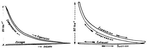
FIG. XIV.—16. Compression Diagram from Engine with cold walls.
