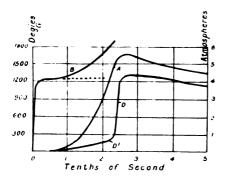
FIG. X.--1. Curve representing pressurerise on combustion (Hopkinson's experiments).
