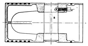
FIG. XIII.---33. Piston for single-acting Engine.
