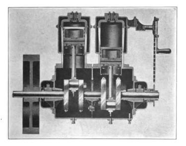
FIG. VI.-10. Section through Gardner (enclosed) vertical Engine.
