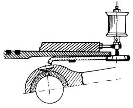
FIG. X.-40. Piston-pin Lubricator.
