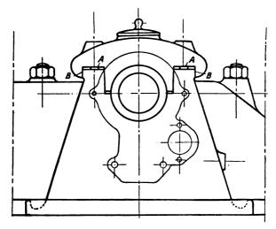
FIG. XII.-25. Bearing with Socket Cap.
