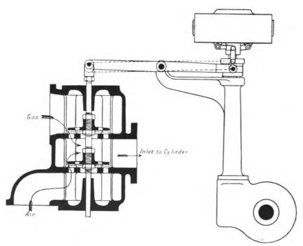
FIG. XI.-12. Westinghouse Air and Gas Throttle Governor.
