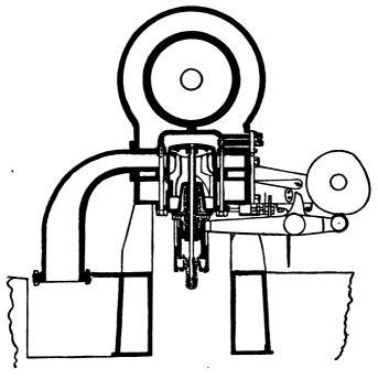
FIG. XIII.--67. Sargent combined Inlet and Exhaust Valve.
