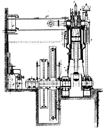
FIG. VI.-2. Sectional elevation of Diesel Engine.
