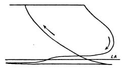
FIG. XIV.--28. Resistance Diagram showing Scavenging by Fluid Inertia.
