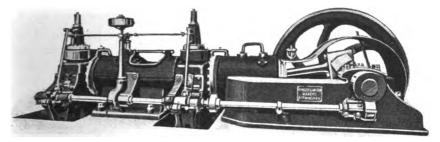
FIG. V.-9. Two-cylinder, tandem, single-acting, four-cycle Kynoch Engine.
