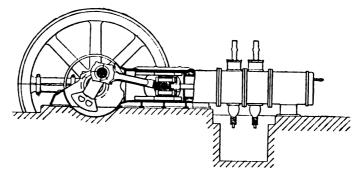
FIG. IV.-15. Dingler Gas Engine, part sectional elevation.
