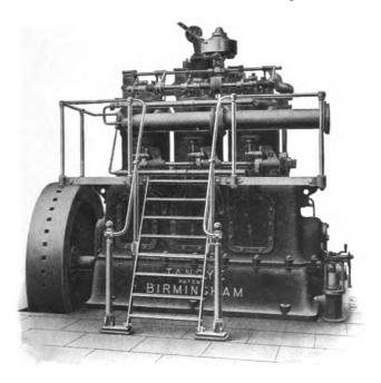
FIG. VI.-18. Three-cylinder, Tangye vertical Engine.
