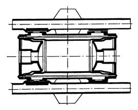
FIG. XII.-52. Section of Cylinder, Cockerill.
