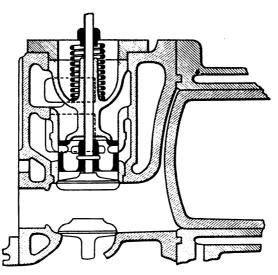
FIG. XII.-- 76. Combustion Chamber of Nürnberg Engine.
