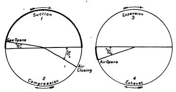
FIG. XV.-16. Diagram of Valve Setting showing "lead" and "lag" of Air Inlet Valve.
