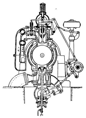
FIG. XL. 32. Governing Device, Otto-Deutz double-acting Engines.
