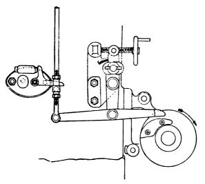
FIG. X.-18. Magneto mechanism, Tangye.
