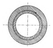
FIG. XII,-18. White-metal lined Bearing after cooling.
