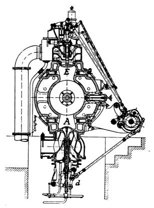
FIG. XI.-36. Governing Device, Otto-Deutz double-acting Engines.
