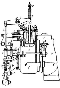
FIG. IV.—9. Hornsby-Stockport governing mechanism (variable admission).
