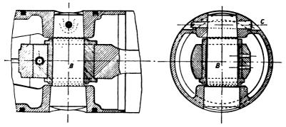
FIG. XIII.-34. Method of securing Piston Pin by Cotter.
