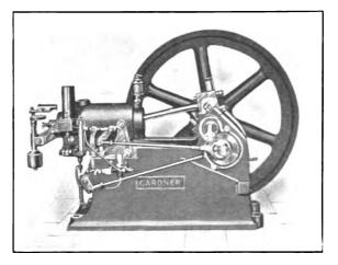
FIG. XIII.-74. Valve Gear of 12 H.P. Gardner Oil Engine.
