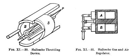
vary the quality and the quantity, and enters, of course, into the fourth class. It consists of a cylindrical box, fitted in the prolongation of the gas and air pipe. In this box is a throttling device S, Fig. XI.—30,
