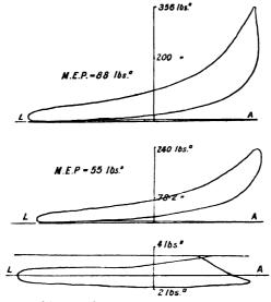
FIG. XV.-36. Diagrams from 600 H.P. Crossley Tandem Gas Engine.
