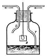
FIG. XIV.--29. Experiment to determine proportion of Carbon Monoxide in Exhaust Gases.
