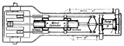
FIG. VIII.-10. Diagram of Oechelhäuser Engine.
