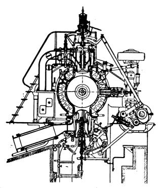
FIG. XI.-33. Governing Device, Otto-Deutz double-acting Engines.
