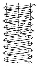
FIG. XIII.-81. Cylindrical Coiled Spring.
