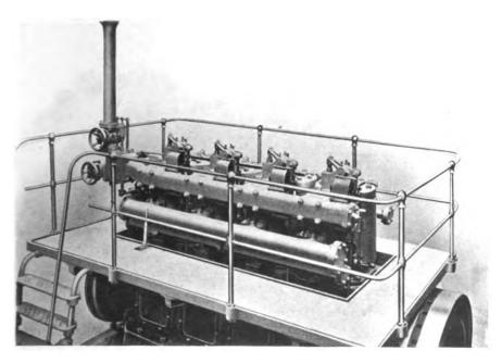
FIG. VI.-14. Cylinder-heads and valve gear, Campbell vertical Engine.
