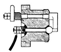
FIG. X.-9. Section through Sparking Plug (Winterthur).
