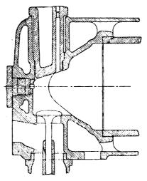
FIG. XII.—71. Form of Combustion Chamber, Tangye (old type).
