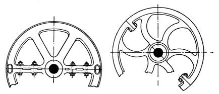
FIG. XIII.-S. Fly-wheel Rim Couplings. FIG. XIII.-9. Fly-wheel Rim Couplings.
