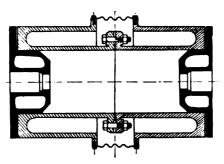
FIG. XII.-54. Section of Cylinder, Snow Steam Pump Works.
