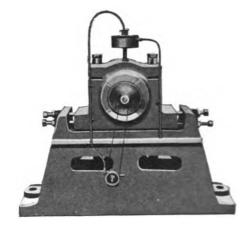
FIG. XII.—30. Hornsby Outer Bearing and special Oiling Device.
