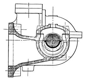
FIG. XII.-31. Cam-shaft Bracket and Ring Oiling Bearing.
