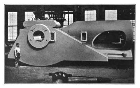
FIG. XII.-10. Frame of 5,400 H.P. Engine (Snow Steam Pump Works).
