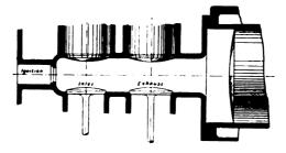
FIG. XIL: -74. Faultily designed Valve Chamber.
