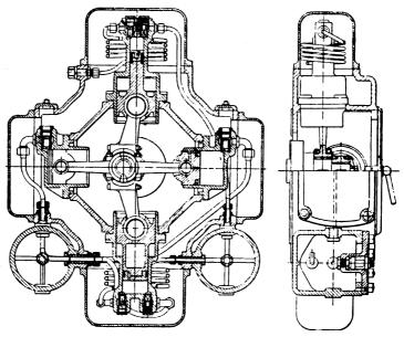
FIG. VI.-7. Section through Reavell Quadruplex Compressor.
