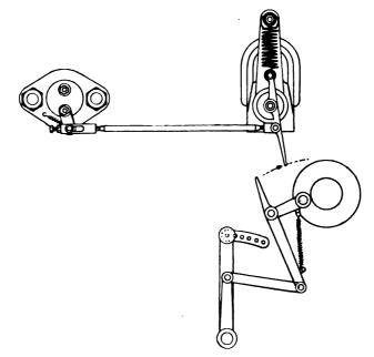
FIG. X.-17. Magneto mechanism, D. Stewart & Co.
