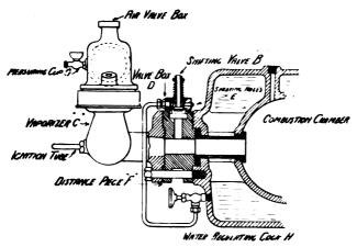
FIG. X.-30. Tangye Oil Engine with water injection device.
