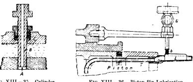
FIG. XIII.—35. Cylinder Lubrication Tube.
