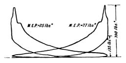
FIG. X.—49. Indicator diagram from double-acting Deutz Engine.
