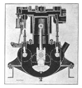
FIG. VI.-11. Transverse section, Gardner (enclosed) vertical Engine.
