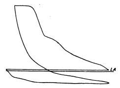
FIG. XIV.-18. Resistance Diagram from throttle-governed Engine, light load.
