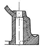
FIG. XII.—16. Boss for Foundation Bolt, with Solid Sheathing.
