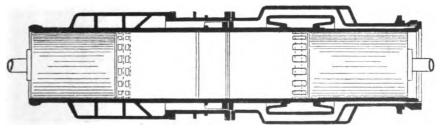
FIG. XII.-37. Section of Cylinder, Oechelhäuser Engine.
