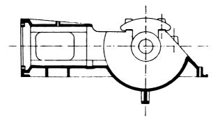
FIG. XII.--6. Frame suitable for various Cylinder Combinations (Reichenbach).
