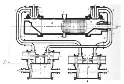
FIG. VIII.-6. Diagram showing Method of Governing (Koerting Engine).
