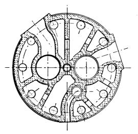
FIG. VI.-4. Section of Cylinder Cover (Diesel Engine).
