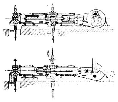
Fig. V.-10. Two-cylinder, tandem, single-acting, four-cycle Winterthur Engine.
