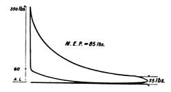
FIG. X.- 48. Indicator diagram from Engine served with town gas.
