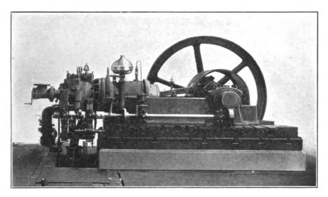
FIG. IV .--- 20. Otto-Deutz. single-cylinder, four-cycle Engine.
