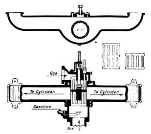
FIG. XI.-13. Alberger Piston Throttle Valve.
