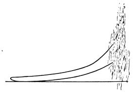
FIG. XIV.-21. Indicator Diagram showing Explosion in Indicator Tube.
