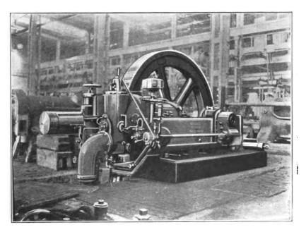
FIG. IV.-29. Nürnberg 60 H.P. single-acting, four-cycle Engine.
