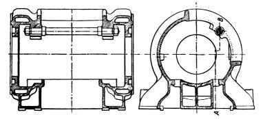
FIG. XII.-58. Intermediate casting or distance piece, Koerting.
