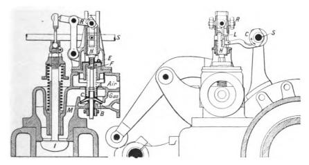
FIG. XI.-47. Snow Steam Pump Co.'s Governing Device.
