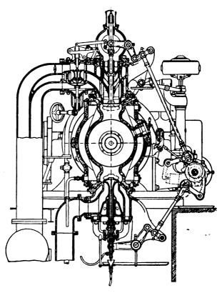
FIG. XI.-34. Governing Device, Otto-Deutz double-acting Engines.
