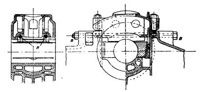
FIG. XII.—26. Transverse Section. FIG. XII.—27. Elevation. Main Bearing Construction of 5,400 H.P. Engine (Snow Steam Pump Works).
