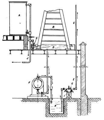
FIG. X.-34. Water circulation with cooling apparatus (visible outlet).
