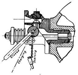
FIG. X.-45. Tangye compressed air Starting Valve.
