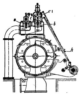
FIG. X1.--37. Governing Device, Otto-Deutz double-acting Engines.
