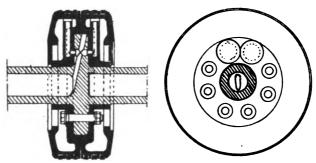
Cockerill Piston and Rod Coupling. FIG. XIII. -53.
