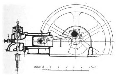
FIG. X.- 36. Water circulation for small engine cylinders.
