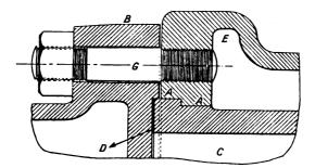
FIG. XII.-33. Detail of Joint between Liner, Jacket, and Breech Casting.
