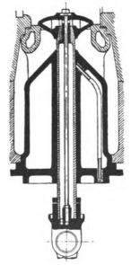
FIG. XIII.—63. End view of Exhaust Valve Lever, Koerting.
