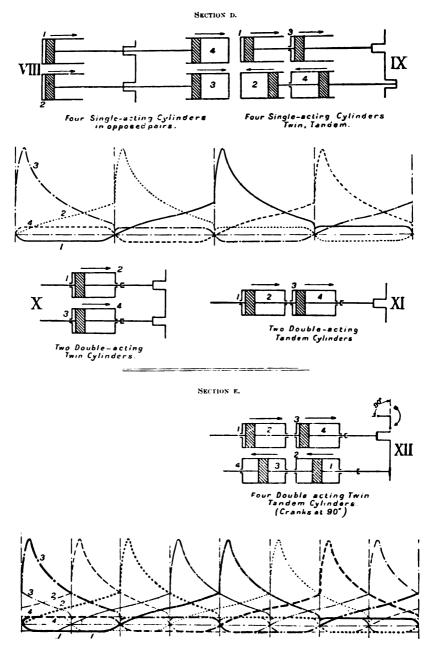
FIG. V.- -5. Characteristic features of various cylinder combinations with relative frequency of impulses (four-cycle engines).
