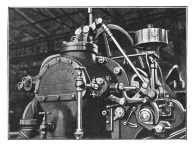
FIG. IV.—2. Olds Gas Power Co.'s 65 B.H.P. Engine, 164 inches diameter by 20 inches stroke, developing 85 H.P. on brake test at 215 revolutions per minute.
