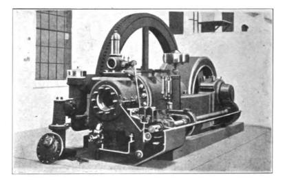
FIG. IV.-24. Koerting four-cycle, single-acting Engine.
