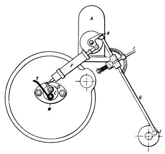
FIG. X.-8. Diagram of magneto low-tension ignition device (Winterthur).
