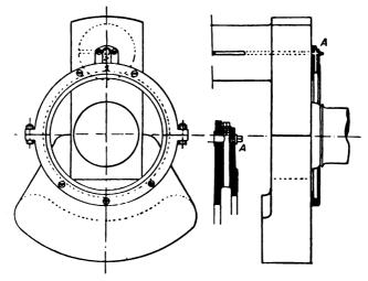
FIG. X.-39. Crank-pin Lubricator.
