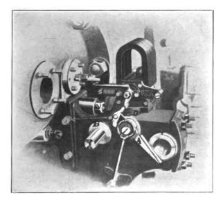
FIG. X.-19. Magneto mechanism, Olds Power Co.
