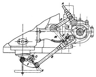
FIG. XIII.-71. Valve Gear with single Cam.
