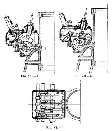
Reversing Mechanism of Gasmotoren Fabrik Deutz Marine Gas Engine.
