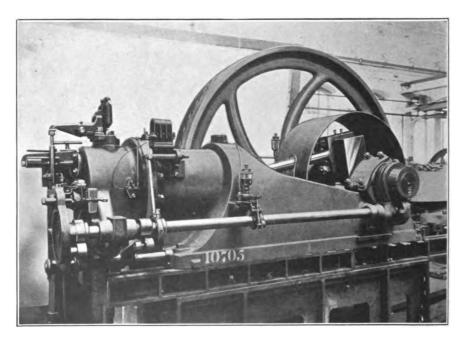
FIG. XIII.--73. Valve Gear of medium power Hornsby-Stockport Engines.
