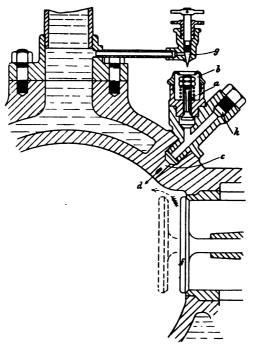
FIG. X.-29. Crossley Gas Engine cylinder with water injection device.
