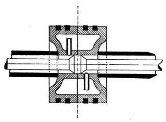
FIG. XIII.-57. Snow Steam Pump Works Piston and Rod.
