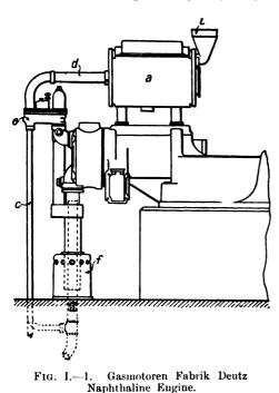
equal, at 59° F., 3½ times that of petrol and 2½ times that of ethyl alcohol. It burns completely away without residue, and, when properly mixed with air, gives a very hot blue flame which is peculiarly steady.
