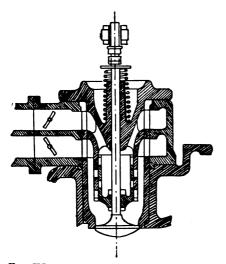
FIG. XI.—10. Governing by variable volume : mixture throttled by separate Butterfly Valves.
