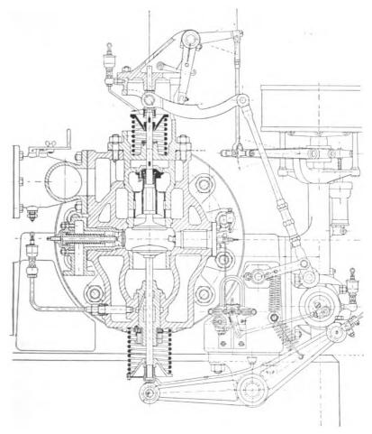
FIG. XII.-77. Section of Combustion Chamber, Gasmotoren Fabrik Deutz.
