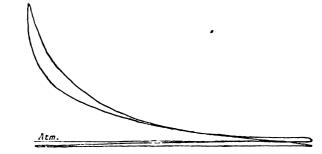
FIG. XIV.-15. Compression Diagram showing loss on Expansion of Charge.
