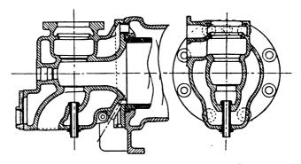
FIG. X11.—78. Longitudinal section. FIG. X11.—79. Transverse section. Form of Combustion Chamber.
