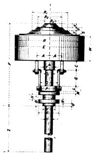
FIG. XIII,--77. Vertical Spindle Governor and Dash-pot.
