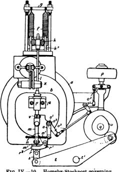
FIG. IV.—10. Hornsby-Stockport governing mechanism (variable admission).
