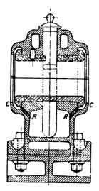
FIG. X11.—29. Outer Bearing and Sole Plate.
