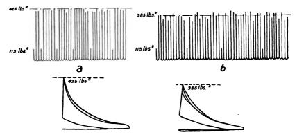
FIG. XV.--26. Records and Diagrams showing variations due to combined exhaust connections.
