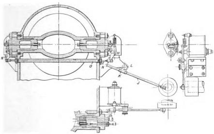
FIG. X. -- 23. Magneto mechanism, National.
