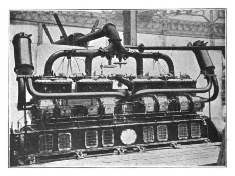
FIG. VII .-- 8. Koerting two-cycle, multi-cylinder Engine, for Submarine Vessels.
