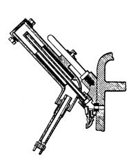
FIG. X.—6. Ignition device with metallic tube.
