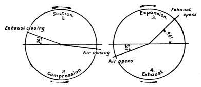
WIG. XV.-10. Diagram of Valve Setting to encourage Scavenging by Fluid Inertia.
