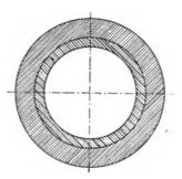
FIG. XII.—17. White-metal lined Bearing before cooling.
