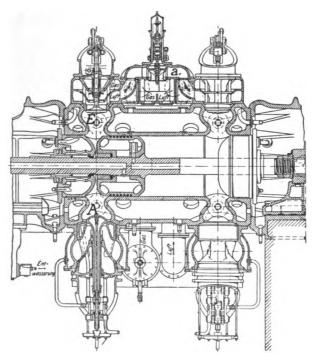
FIG. XI.-35. Governing Device, Otto-Deutz double-acting Engines.
