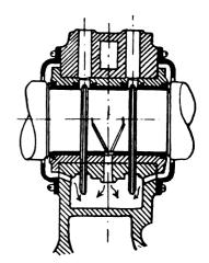
FIG. XII.—22. Shaft in Bearing, with Oiling Ring.
