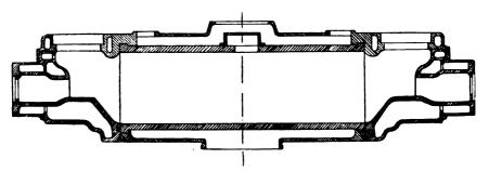
FIG. XII.-38. Section of Cylinder, Koerting Engine.
