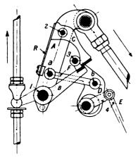
FIG. VIII.—12. Governor Trip Gear, Occhelhäuser Engine.
