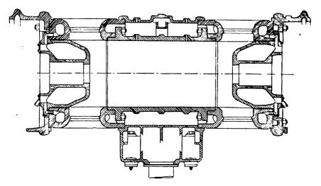
FIG. XII.-46. Section of Cylinder, Gasmotoren Fabrik Deutz.
