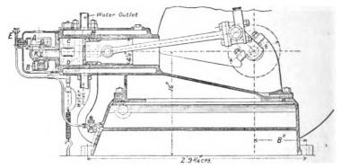
FIG. IV.-8. Britannia Engineering Co.'s Petroleum Engine.
