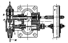
FIG. VI.—6. Section through Fuel Pump, showing automatic Governing Device (Diesel Engine).
