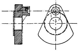
FIG. X111.-20. Side Crank. Snow Steam Pump Works.
