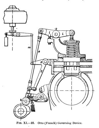
Co., similar to that used by the French Otto Co., Fig. XI.—22. The main lever Ll is fulcrumed at 2 with a rod a, resting at its lower end on a curved link b.
