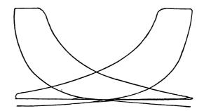
FIG. IX. -4. Representative indicator diagrams taken with "light" springs from Sargent Gas Engine.
