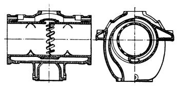
FIG. XII.-39. Section of Cylinder, Koerting type, Gutehoffnungshütte.
