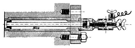
FIG. X.-25. High-tension Sparking Plug for Lodge ignition system.
