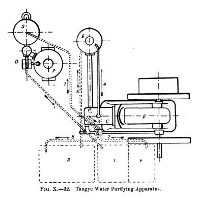
tank (R) from which it is pumped through the pipes (6) and (7) to the scrubber, in which it again meets and cools the gas and commences once more the "cycle" of purification. The water used in the vaporiser is necessarily irrecoverable, because it is transformed into vapour whilst passing through the mass of incandescent fuel, and combined with the latter to form hydrogen and carbon monoxide.
