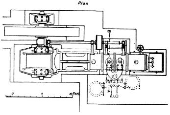
FIG. IV.-16. Dingler Gas Engine, plan.
