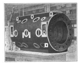
FIG. XII.-55. Cylinder Casting, Allis Chalmers Co.
