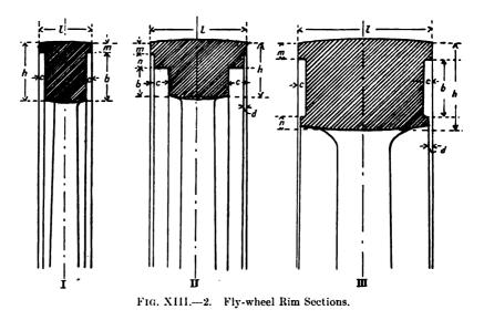
and breadth are necessarily a function of the selected shape. For the purpose of calculation three simple forms have been adopted, as shown
