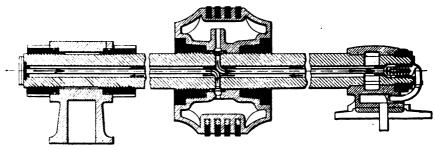
FIG. X111.-52. Reichenbach Piston, Rod, and Crossheads.
