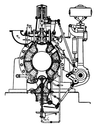
FIG. IV.-7. Transverse section of Struthers Wells Co.'s Tandem Engine.
