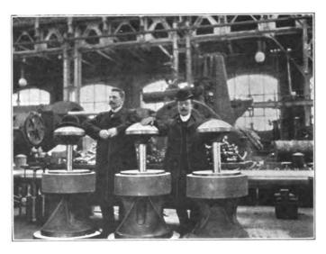
FIG. XIII. 65. Three Exhaust Valves for 2,000 H.P. Nürnberg Engine.
