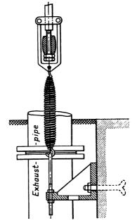
FIG. XIII.—80. Tension Spring on Exhaust Valve.
