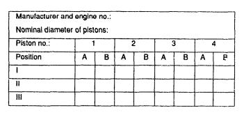
Clean the bearings thoroughly and tighten them again with the torque wrench. Use the micrometer to measure the bearings at the positions 2-A1, 2-A2, 2-B1, 2-B2. Enter the sizes in the table below. Find the difference between the nominal size and the actual size.
