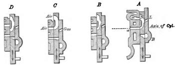
Fig. 43.—Otto Engine—Positions of Ports and Passages. 1876.
