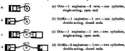
Fig. 33.—Diagram of Single- and Double-Cylinder Explosion Engines.
