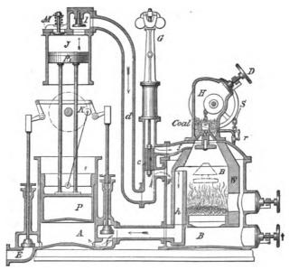
Fig. 157.—Buckett Air Engine—Single Cylinder.
