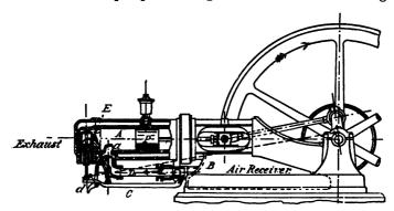
Fig. 92.—Benz Gas Engine—Elevation.
