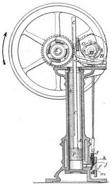
Fig. 9.—Otto and Langen Vertical Engine— Transverse Section. 1866.
