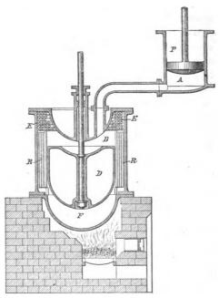
Fig. 159.—First Stirling Engine. About 1830.
