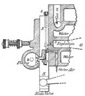
Fig. 21.—Clerk Engine—Ignition Valve. 1880.
