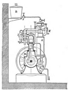
Fig. 147.—Daimler Oil Engine. 1890.
