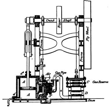
Fig. 6.—Hugon Gas Engine—Vertical. 1862.
