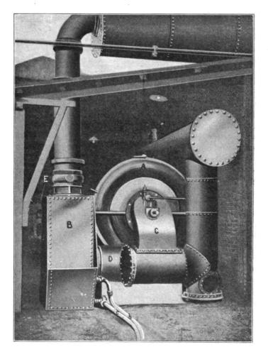
Fig. 110.—Centrifugal Fan for Cleaning Blast-furnace Gases.
