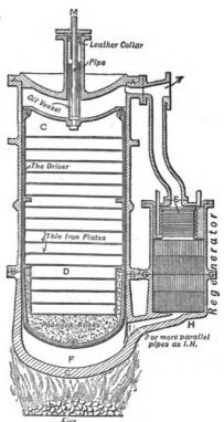
piston up and down in its passage. There is no exhaust, the same air being used continuously, and a closed cycle is thus obtained. This engine presents in a compact form the main principles of Stirling's invention, and illustrates better than any other type of motor the construction of a perfect heat engine. Here we have the source of heat (the furnace), the source of cooling (the refrigerator),
