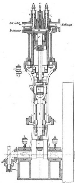
voir L at the side, where Fig. 156.—20 Horse-power Diesel Oil Motor. it is at a pressure of 35 to 50 atmospheres. From thence it passes
