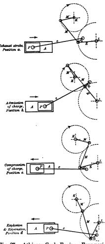
gases and a portion of the fresh compressed mixture up the redhot part of the tube, where they ignited, and spreading back into the cylinder fired the remainder.
