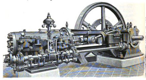
Fig. 80.—Letombe Gas Engine—Double-acting.
