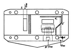
Fig. 39.—Otto Engine—Vertical View of Slide Cover. 1876.
