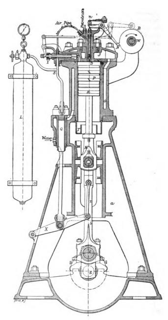
Fig. 155.—20 Horse-power Diesel Oil Motor.
