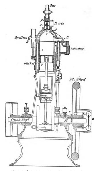
Fig. 94.—Capitaine Gas Engine —Sectional Elevation.
