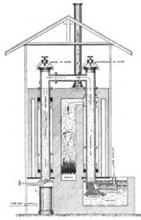
Fig. 109.—Wood Gas Producer—Section (Riché). 1899.
