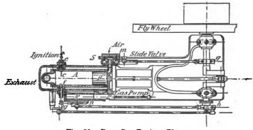
Fig. 93.—Benz Gas Engine—Plan.
