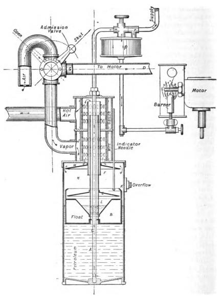
Fig. 148.—Daimler Oil Engine. Vaporiser.
