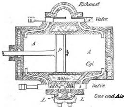
Fig. 4.—Lenoir Engine—Section of Cylinder. 1860.
