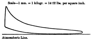
Fig. 106.—Indicator Diagram of 29 H.P. Engine worked with Pierson Suction Producer.
