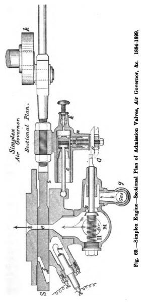
opening at the bottom of the cylinder, communicating with it through the valve S'. The air enters at H, the gas at g, through a pipe at right
