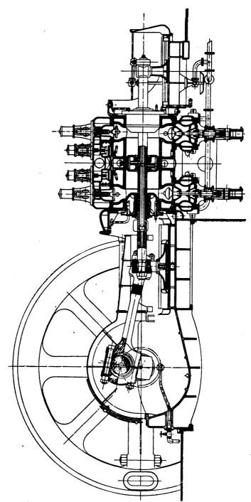
Fig. 86.—Nuremberg Double-acting Engine—Longitudinal Section.
