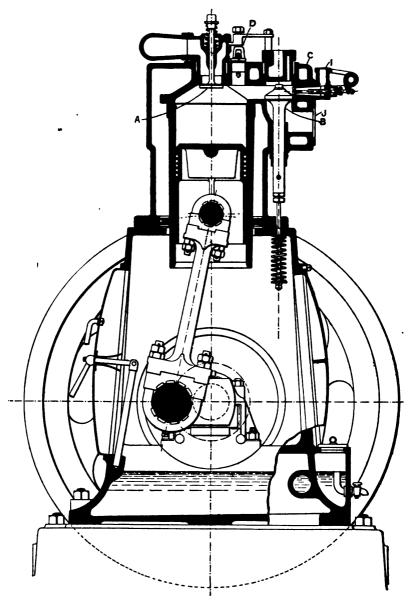
Fig 57.—150-H.P. Four-cylinder Fielding & Platt Engine—Sectional Elevation.
