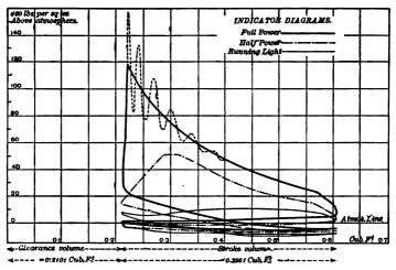
Fig. 135.—Priestman Oil Engine—Indicator Diagram.
