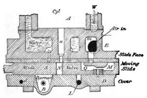
Fig. 37.—Otto Engine, 1876—Sectional Plan of Slide Valve.
