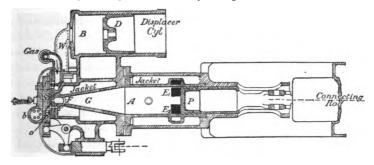
Fig. 20.—Clerk Engine—Sectional Plan. 1880.
