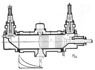
Fig. 84.—Koerting Engine—Section of Cylinder with Diagram.
