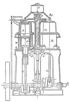
Fig. 130.—Siemens' Regenerative Engine. 1881.
