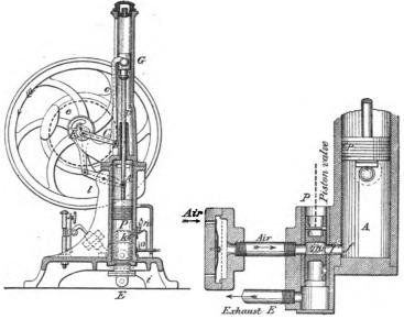
Fig. 14.—Bisschop Engine—Sectional Elevation. 1870.
