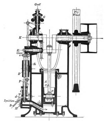
Fig. 91.—Adam Gas Engine—Sectional Elevation. 1888-1899.
