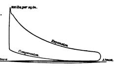
Fig. 151.—Otto-Petroleum Engine. Indicator Diagram.
