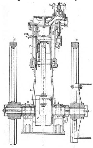
Fig. 154.—Banki Oil Engine—Sectional Elevation.
