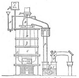
Fig. 126.—Mansfield Oil Gas Producer.
