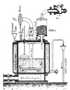
Fig. 150.—Benzine Carburator—Otto Engine.
