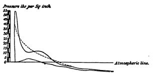
Fig. 13.—Otto and Langen Engine—Indicator Diagram (Clerk). 1866.
