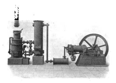
Fig. 107.—Deutz Suction Gas Producer.
