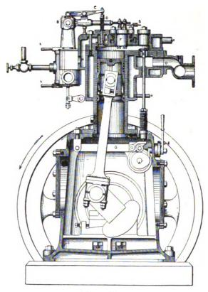
Fig. 59.—Sectional View, Westinghouse Engine.
