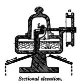
Fig. 45.—Otto Gas Engine— Oiling Apparatus.
