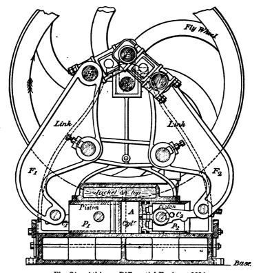
Fig. 24.—Atkinson Differential Engine. 1884.
