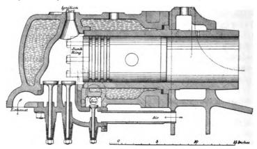
Fig. 125.—Experimental Gas Engine—Burstall's Tests. 1898, 1901.
