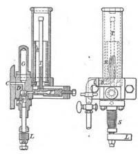
Fig. 46.—Otto Engine—Ignition Tube. 1888.
