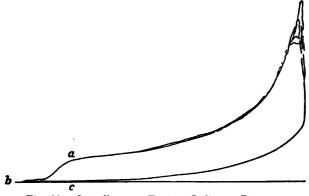
Fig. 89.—Oechelhaueser Engine—Indicator Diagram.
