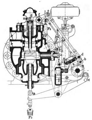
Fig. 87.—Nuremberg Engine—Valve Gear and Governor.
