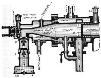
Fig. 19.—Clerk Engine—Sectional Elevation. 1880.
