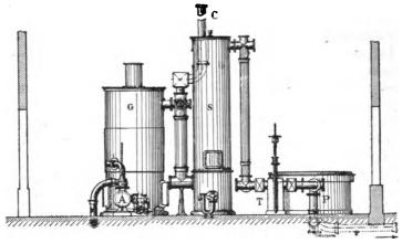
Fig. 102.—Lencauchez Gas Plant—Elevation.
