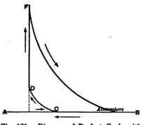
Fig. 121.—Diagram of Perfect Cycle with Compression.
