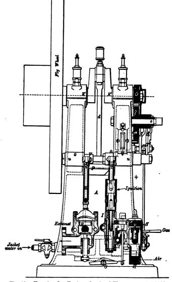
Fig. 81. -Koerting Gas Engine-Sectional Elevation. 1888-1899
