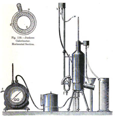
Fig. 120.—Junkers Gas Calorimeter, with Gas Meter, &c.
