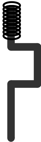
Figure 2: using bent steel rod to rotate drill.
