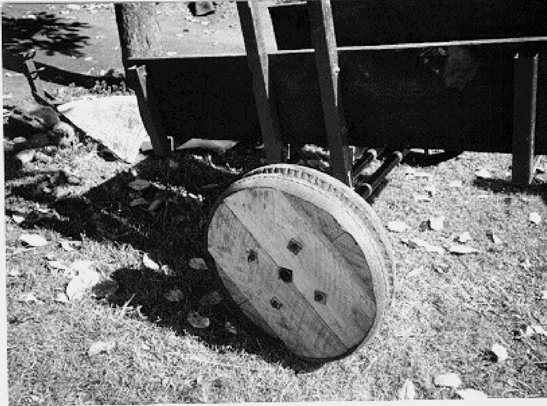
Figure 1: wood wheel for an air pump using old rubber and timber.
