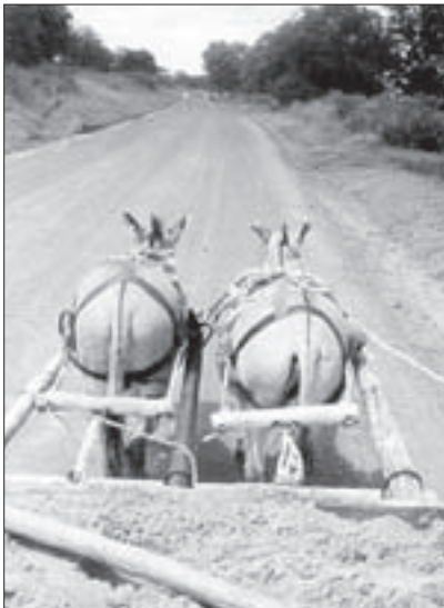
Fig. 34 (above): Vertical load on a single shaft cart well balanced by fitting two extra shafts to minimise pressure on the neck of the donkeys
